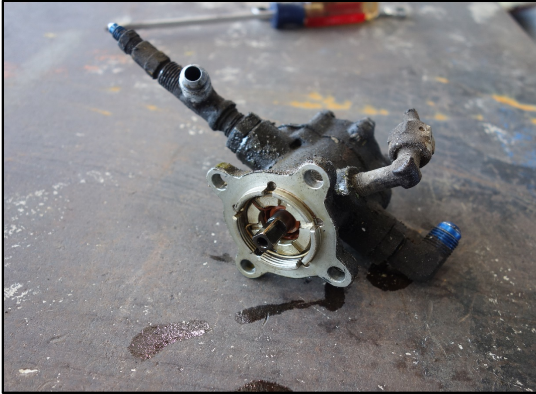
Figure 2: Fuel Pump removed for examination.
