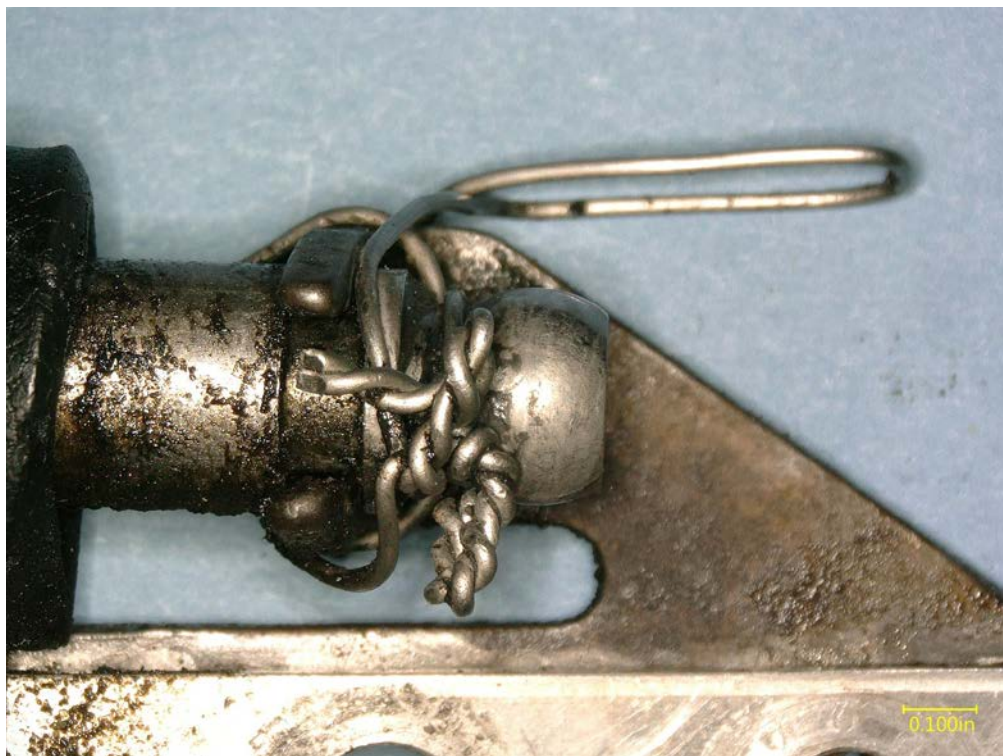
Figure 2: Digital microscope images of the detached ball mount before (top) and after (bottom) cleaning. Safety wire was observed wrapped around the base of the ball mount.
