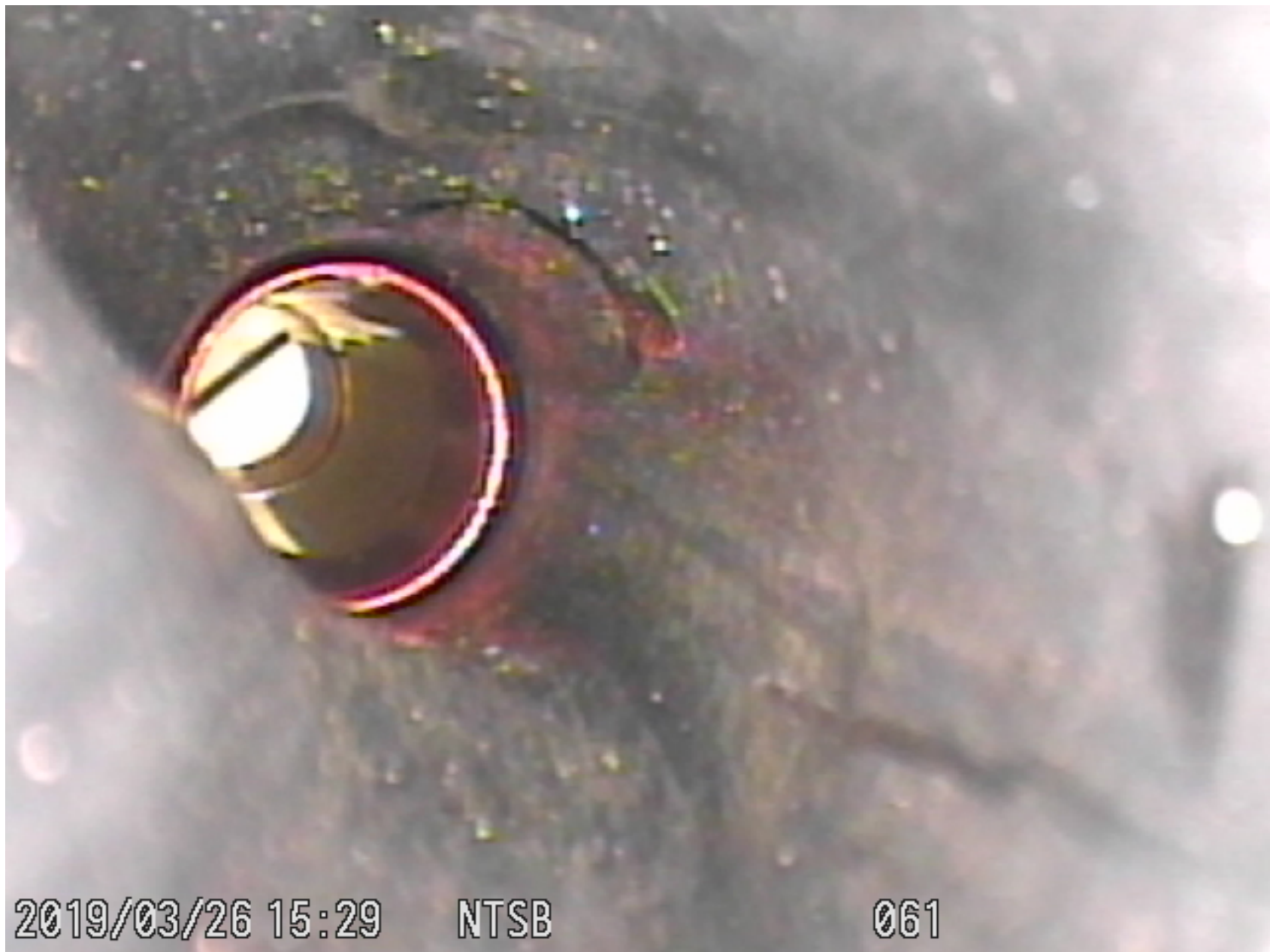
Photo 7 – N46321 Fuel Hose Inner Diameter
