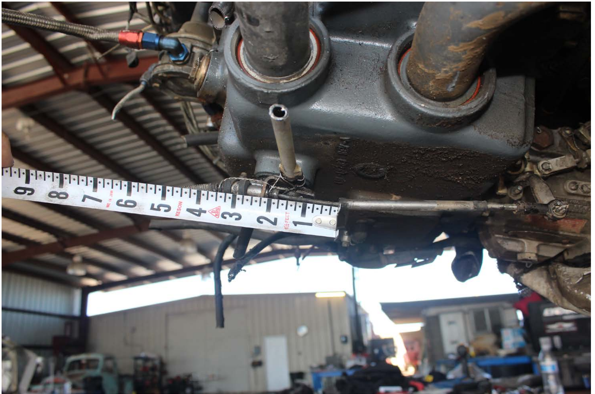
Photo 9 – N46321 Throttle Cable with Detached Throttle Cable Sheath
