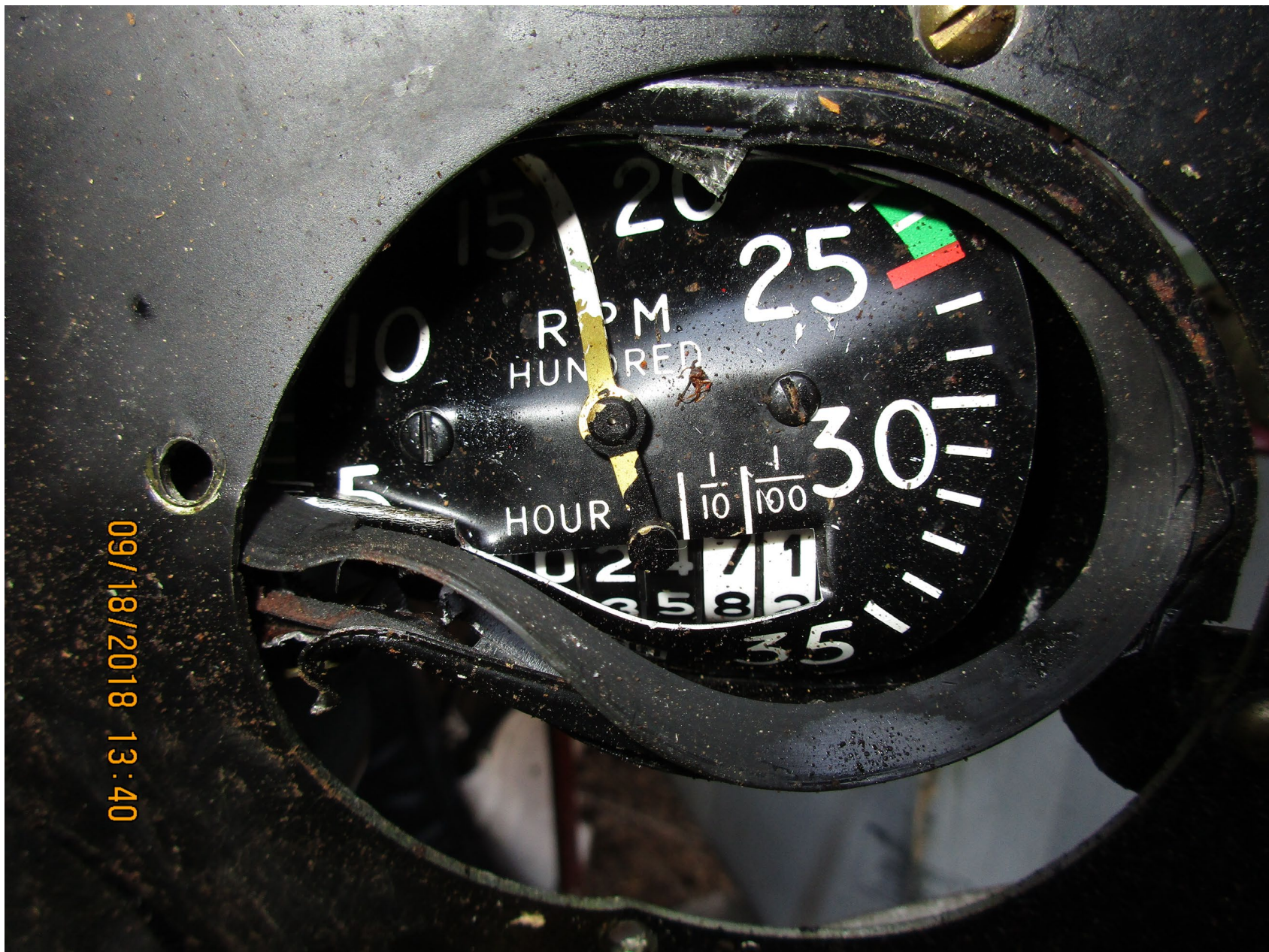
Photo 12 – Hour Meter (Photo Courtesy of FAA)
