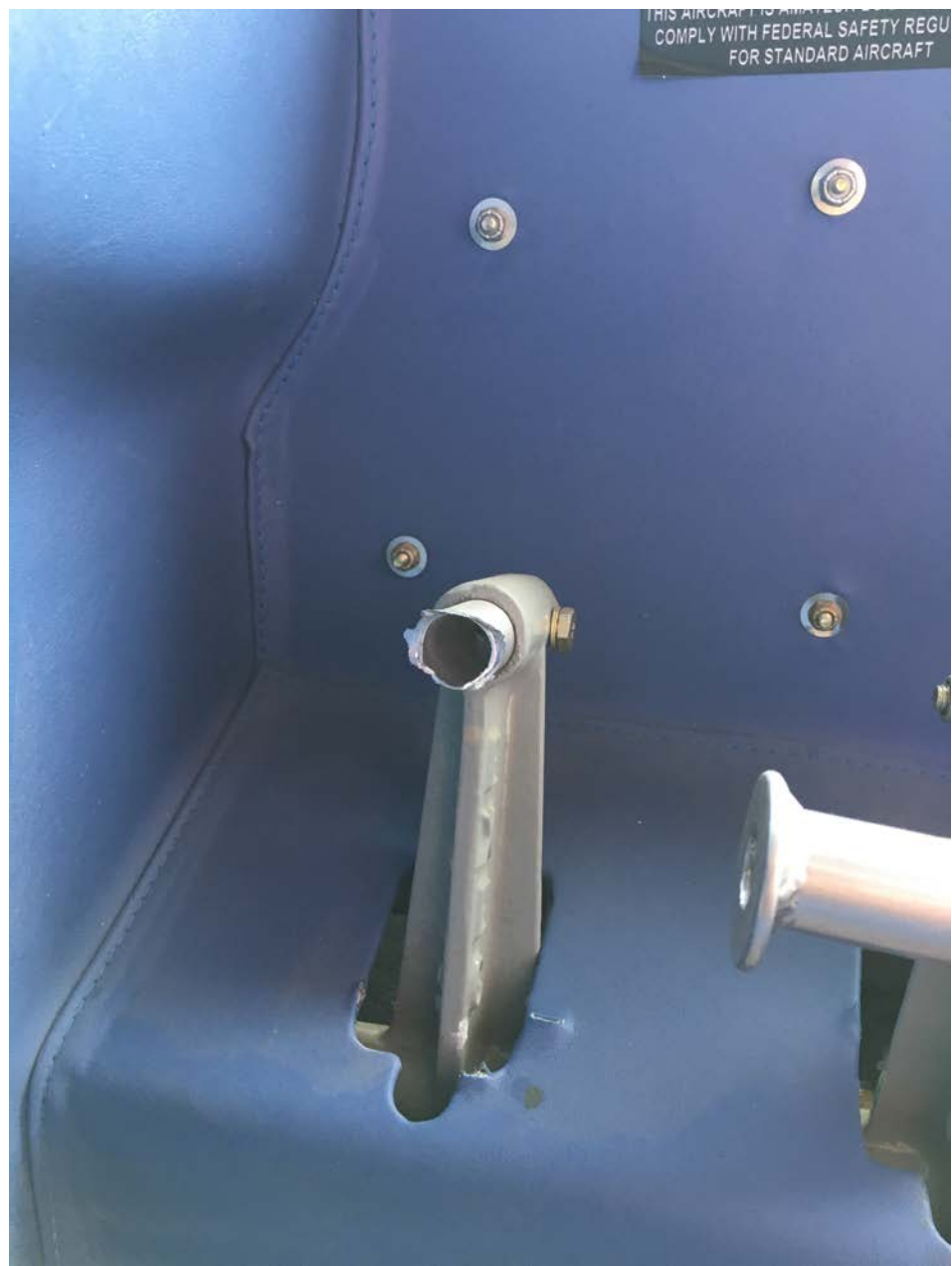
Photo 5 – photo of failed vertical anti-torque pedal
