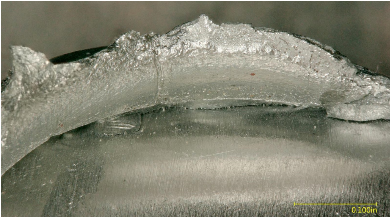
Figure 6 – Closer view of the largest remnant of the fractured joint on the parallel tube.
