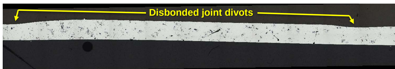
Figure 24 – Bright-field optical micrograph montage of the cross section of the parallel aluminum tube through the fractured joint. Those divots where the filler metal had disbonded from the joint are annotated (~25X, as polished).
