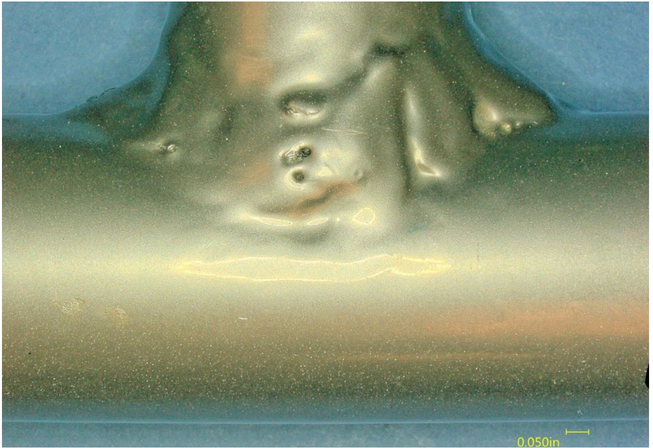
Figure 21 – Closer view of the intact anti-torque tube showing surface porosity.
