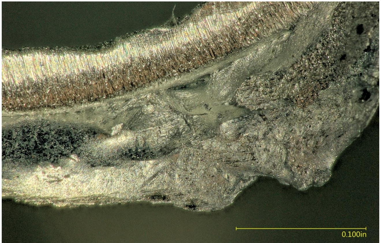
Figure 9 – View of the largest filler metal remnant on the perpendicular tube fracture surface.
