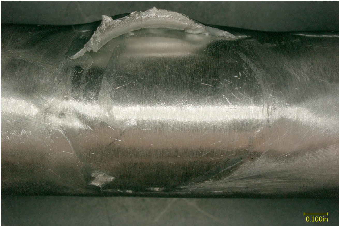
Figure 5 – Closer view of the parallel tube side fracture surface.
