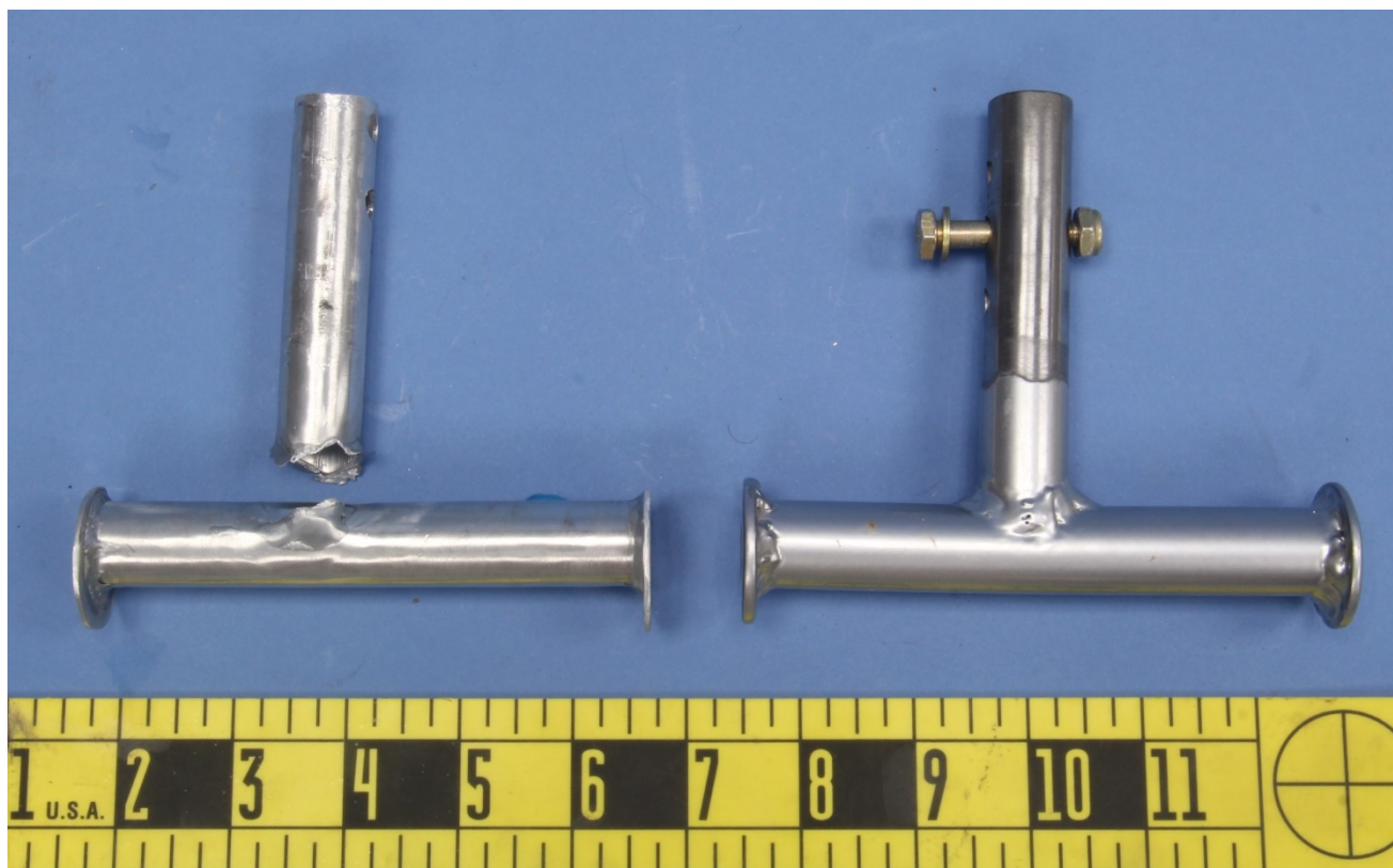
Figure 1 – The anti-torque tubes, as received. The tube on the left had fractured at the joint, whereas the assembly on the right was intact.
