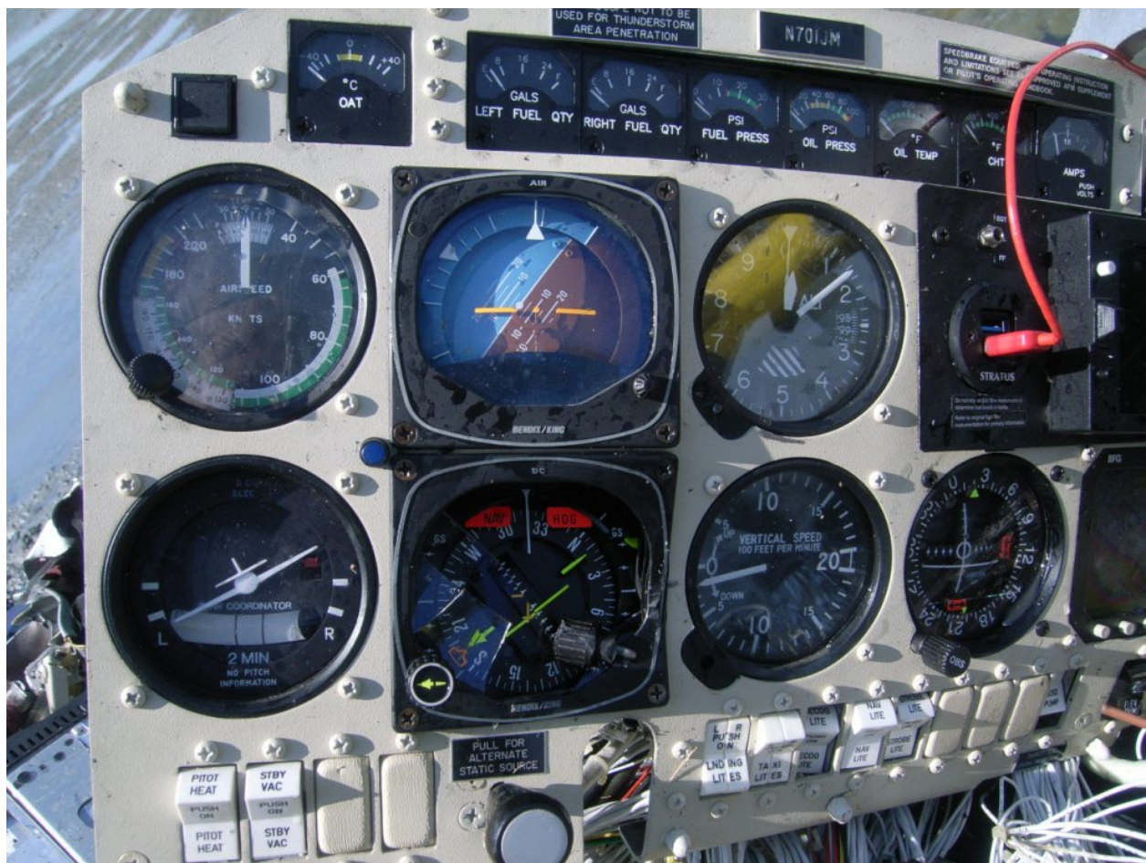
Figure 14 - Left Instrument Panel
