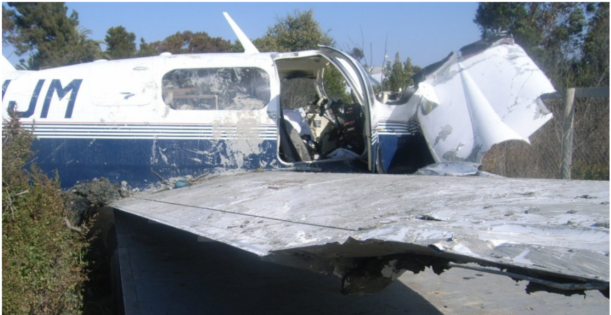
Figure 20 - Right Wing and Flap
