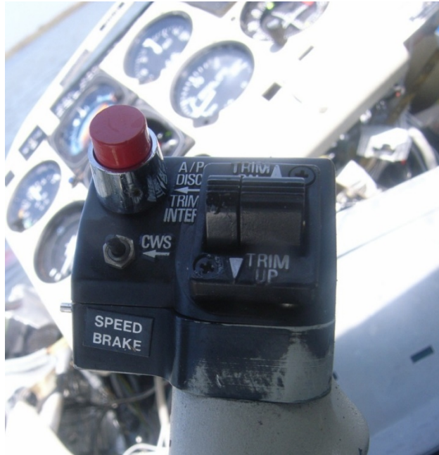
Figure 12 - Pilot's Yoke (Left horn)
