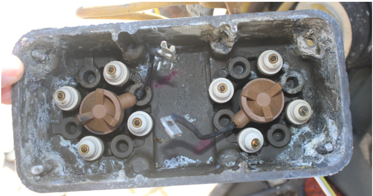
Figure 23 - Opened Magneto (cover)
