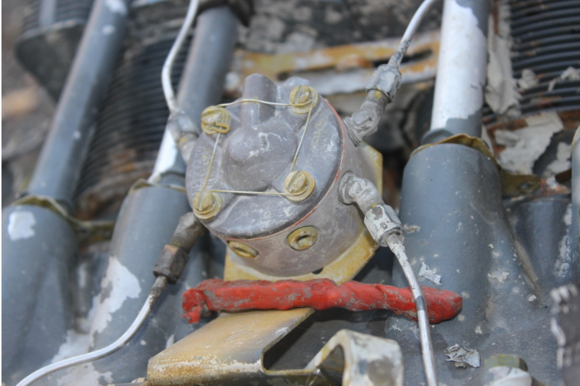
Figure 17 - Manifold Fuel Distribution Valve
