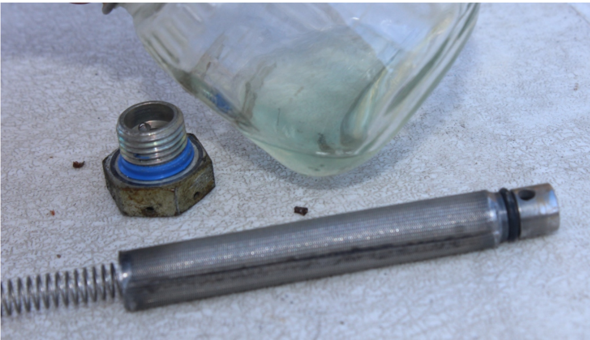
Figure 16 - Fuel Screen and Fuel
