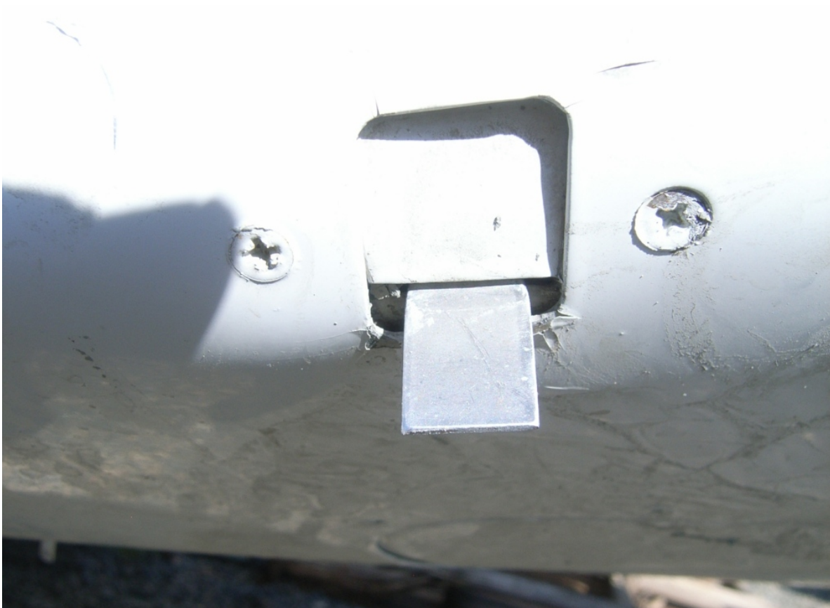
Figure 4 - SWS Vane (in situ)
