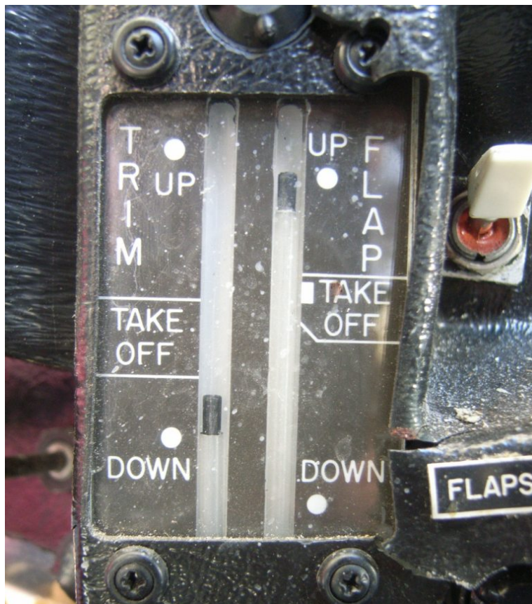
Figure 8 - Pitch Trim & Flap Cockpit Indicators
