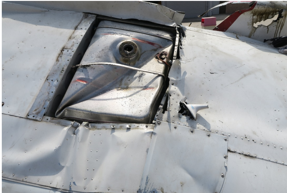
Figure 7: Left Fuel Tank
