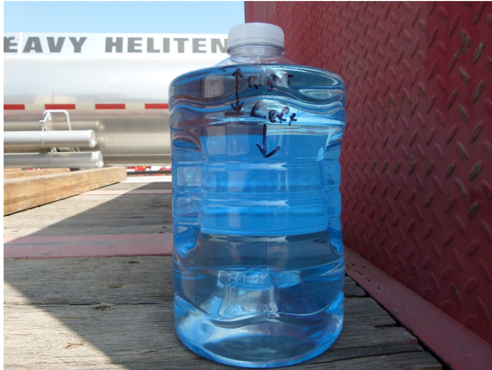
Figure 9: Total Fuel Removed from Airplane
