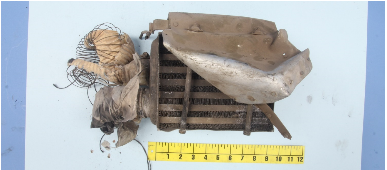
Figure 1 – View of the heat exchanger and surrounding housing and tube, as received.
