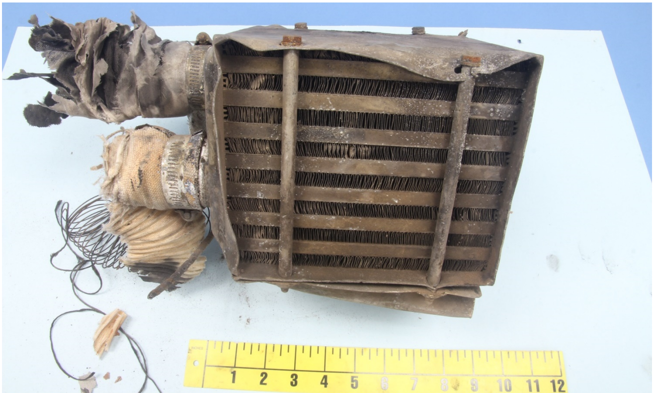
Figure 2 – Side view of the heat exchanger, showing the extent of damage to the assembly, as received.
