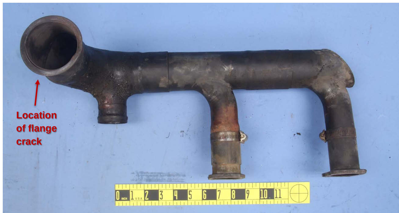
Figure 2 – The exhaust manifold, showing the location of the crack on the output flange.
