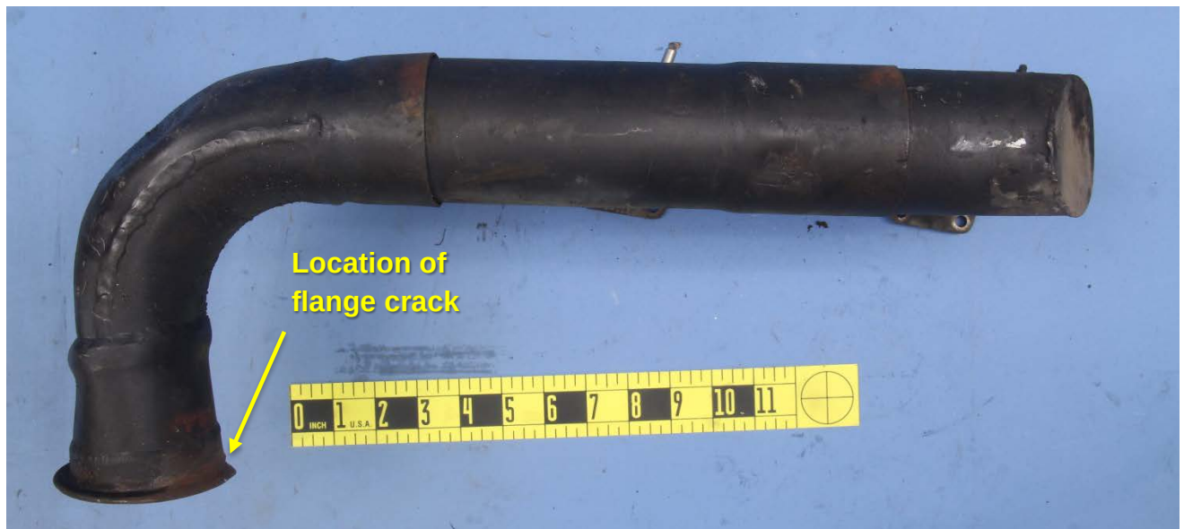
Figure 3 – View of the exhaust manifold, rotated 90° from Figure 2, with the crack location labeled.
