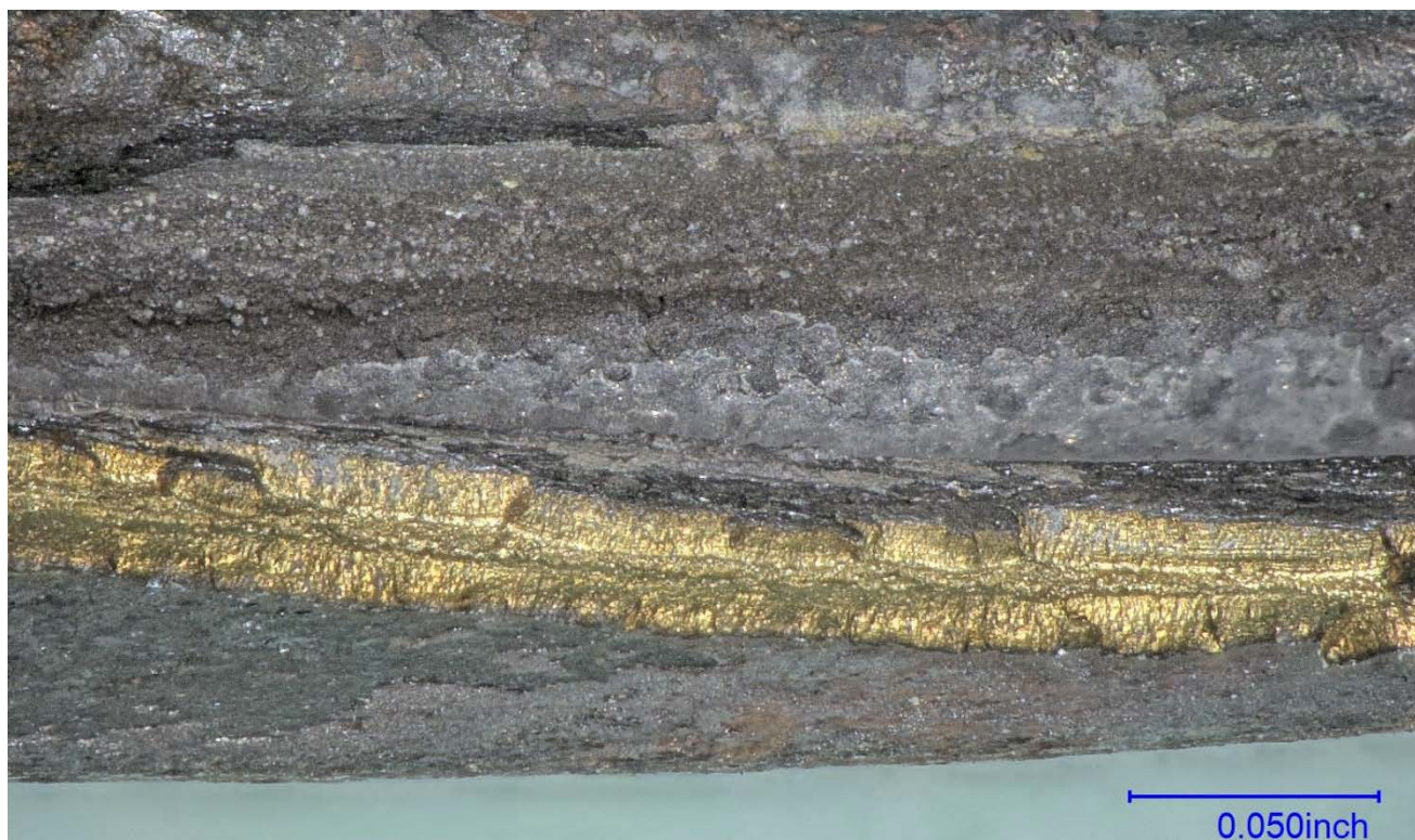
Figure 5 – Closer view of a portion of the opened crack, showing multiple thumbnail cracks and ratchet marks.
