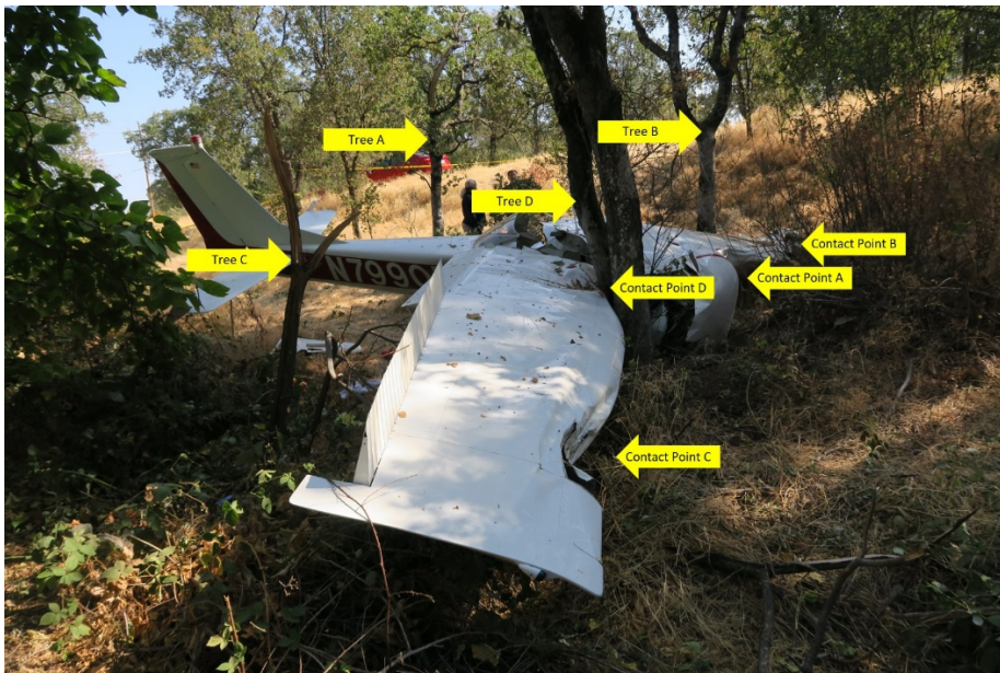
Photo 3. Leading edge contact points and trees with damage.
