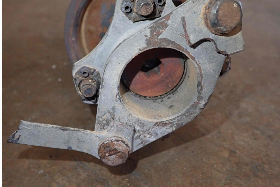
Photo 12 - Flexible Coupling Transmission Side
