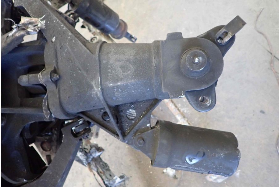
Photo 21 – Blue Blade Pitch Housing
