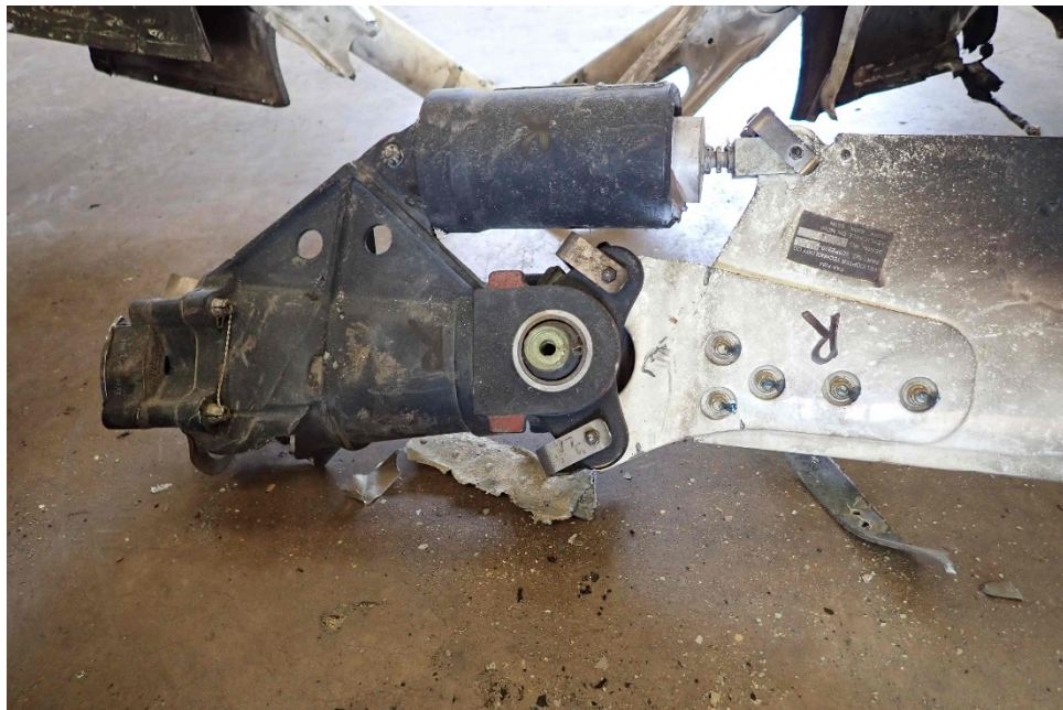
Photo 15 – Red Blade Pitch Housing
