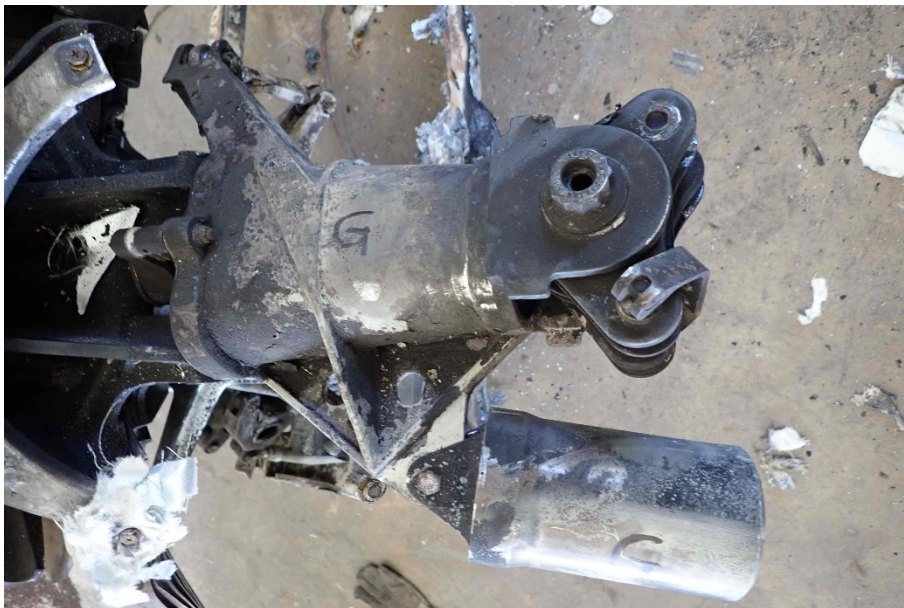
Photo 17 – Green Blade Pitch Housing
