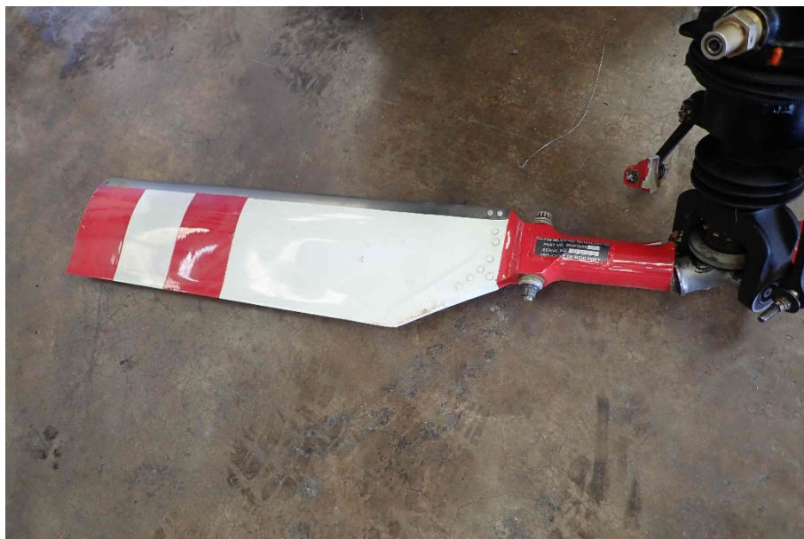
Photo 30 – Tail Rotor Blade
