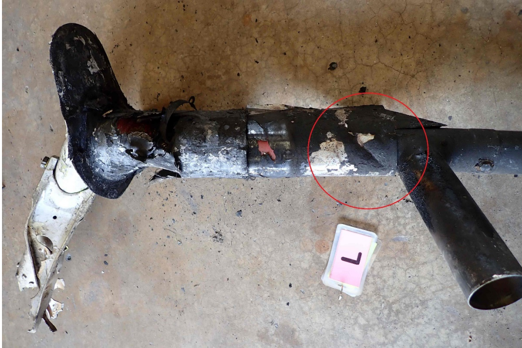
Photo 4 – Left Forward Strut, Upper Fairing
