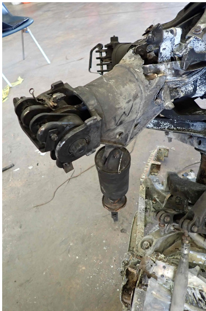
Photo 24 – White Blade Pitch Housing
