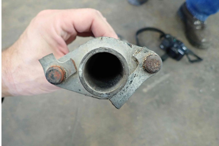
Photo 10 – Flexible Coupling Engine Side
