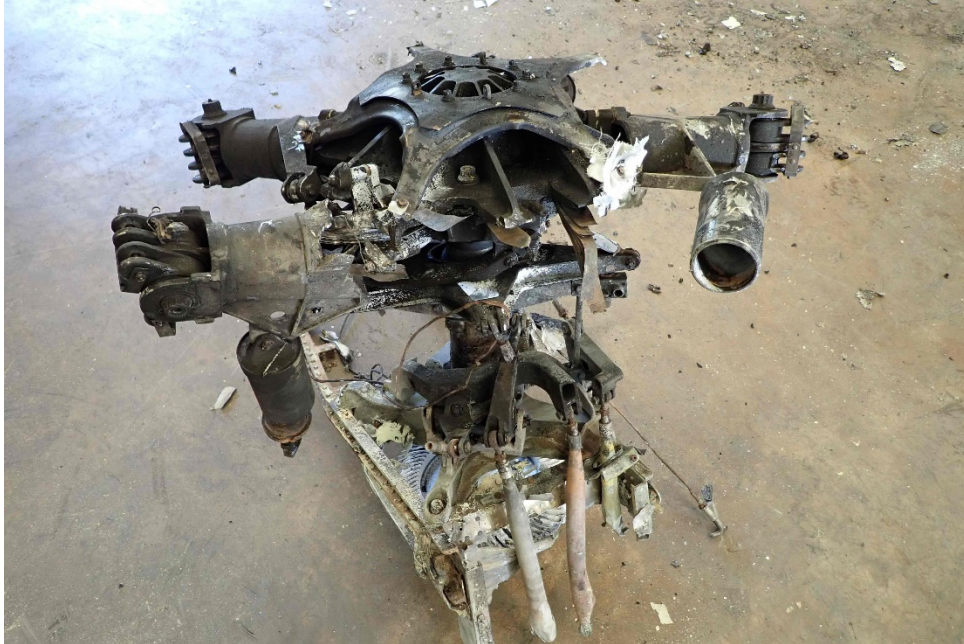
Photo 14 – Main Rotor Hub
