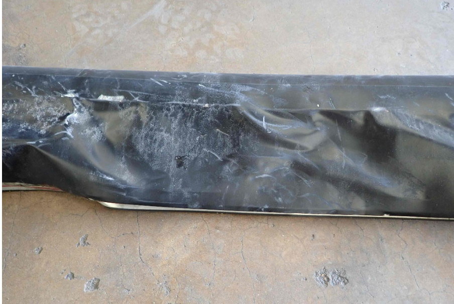
Photo 23 – Blue Blade Damage
