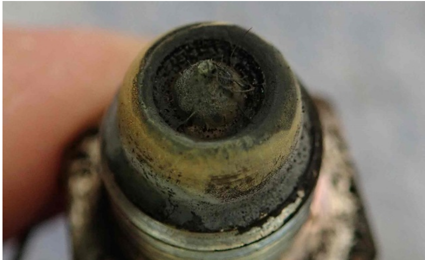
Photo 2 - Gearbox Upper Chip Detector
