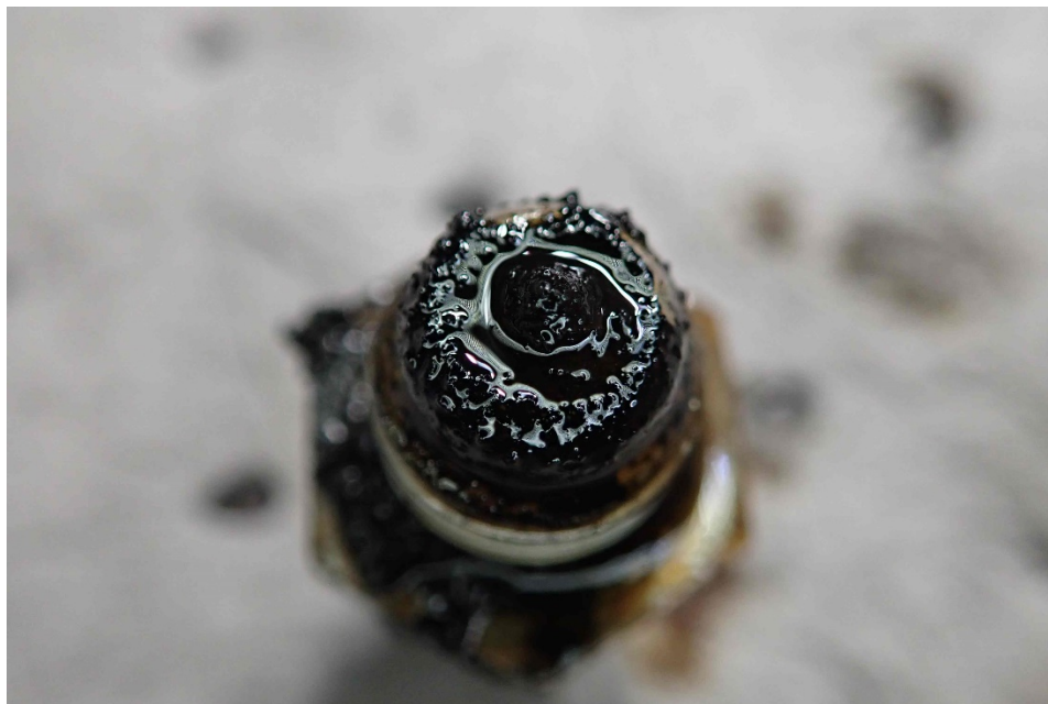
Photo 3 - Gearbox Lower Chip Detector
