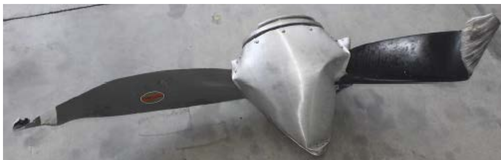
Figure 2 - photo of damaged propeller blades
