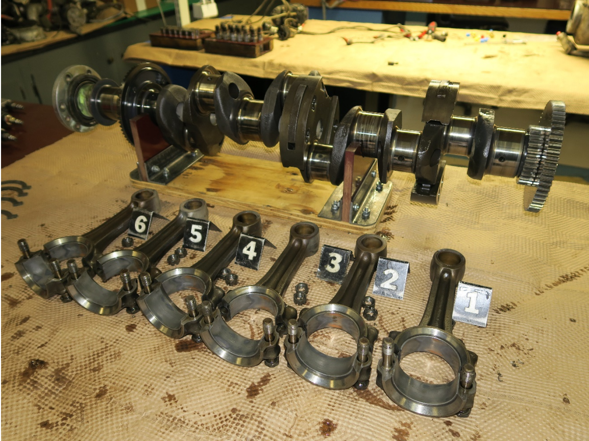
Figure 6: Crankshaft and Bearing Wear
