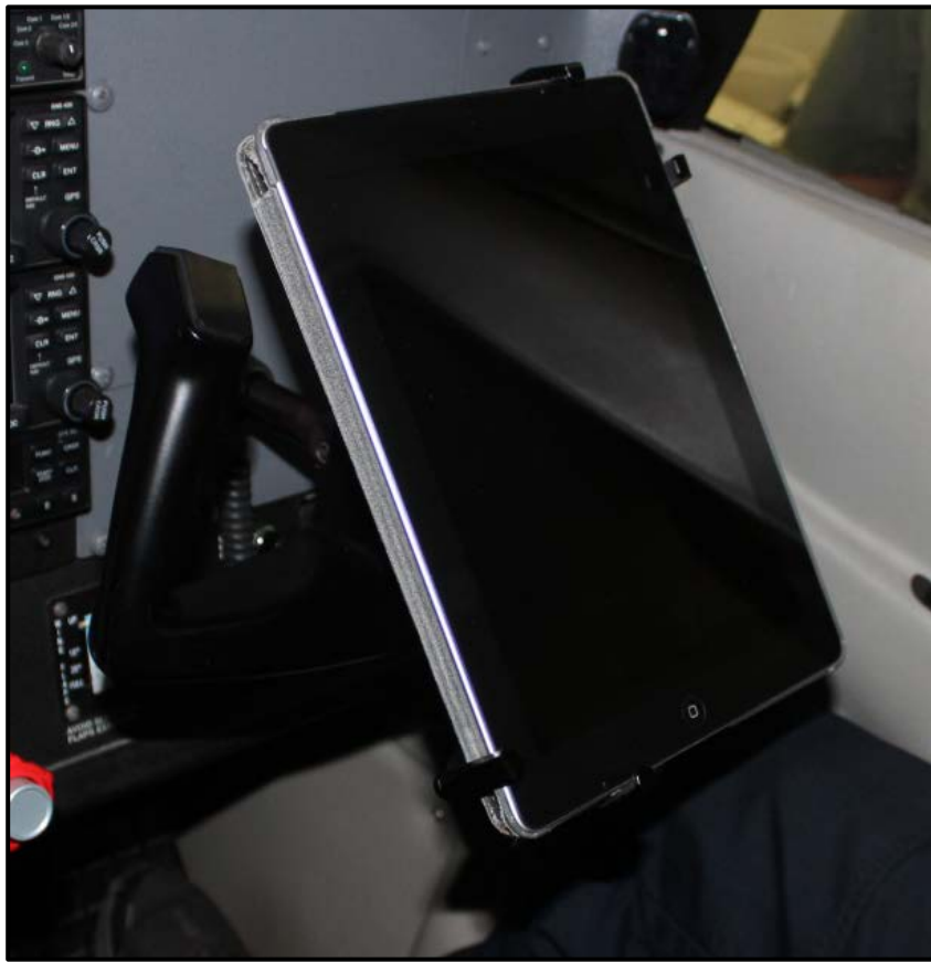
Picture 24: Shown Installed with iPad on an Exemplar (forward)
