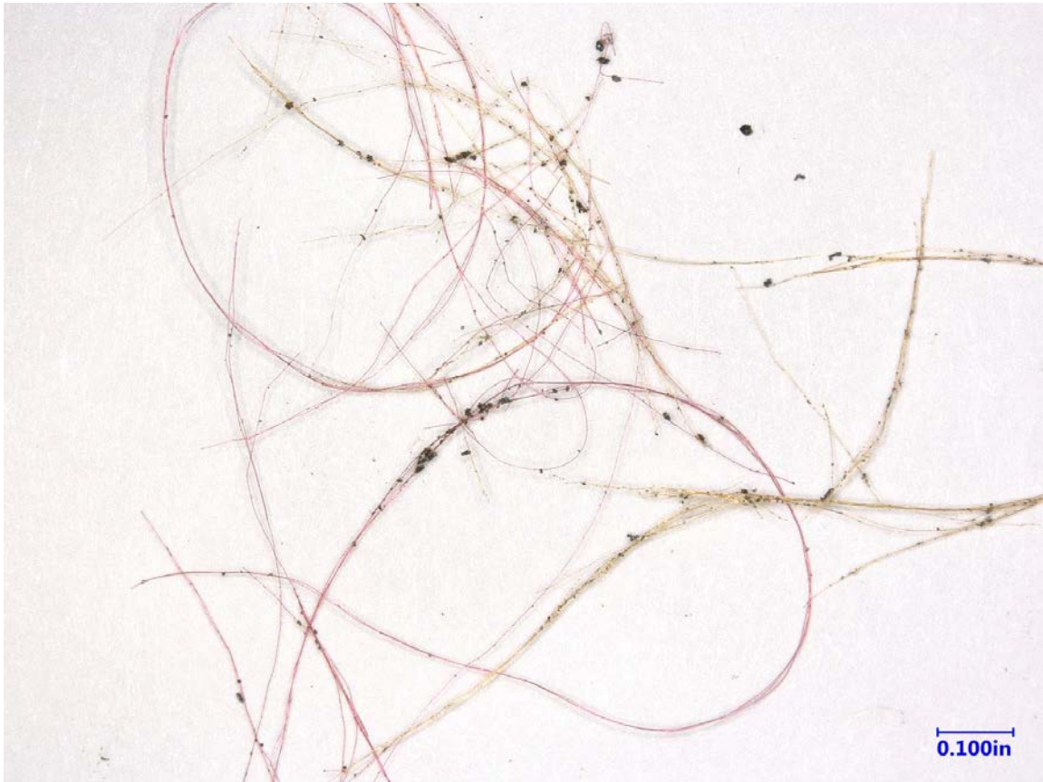
Figure 9: Digital microscope image of red colored and gold colored fibers removed from the left overhead aileron to wing cable.
