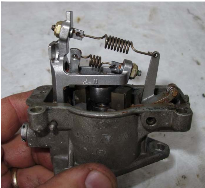
Figure 7 Fuel Control Unit Drive Body
