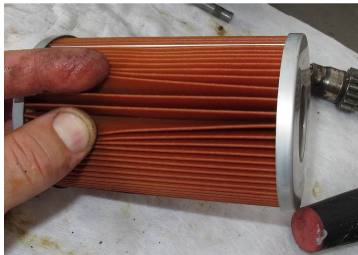
Figure 5 Airframe Fuel Filter Element
