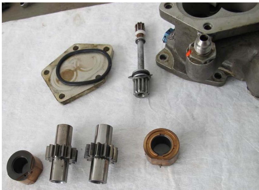
Figure 11 Disassembled Fuel Pump
