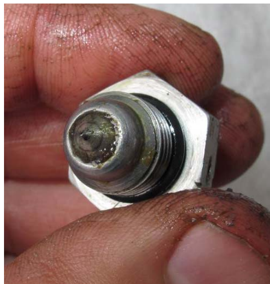
Figure 22 Bottom Magnetic Chip Detector
