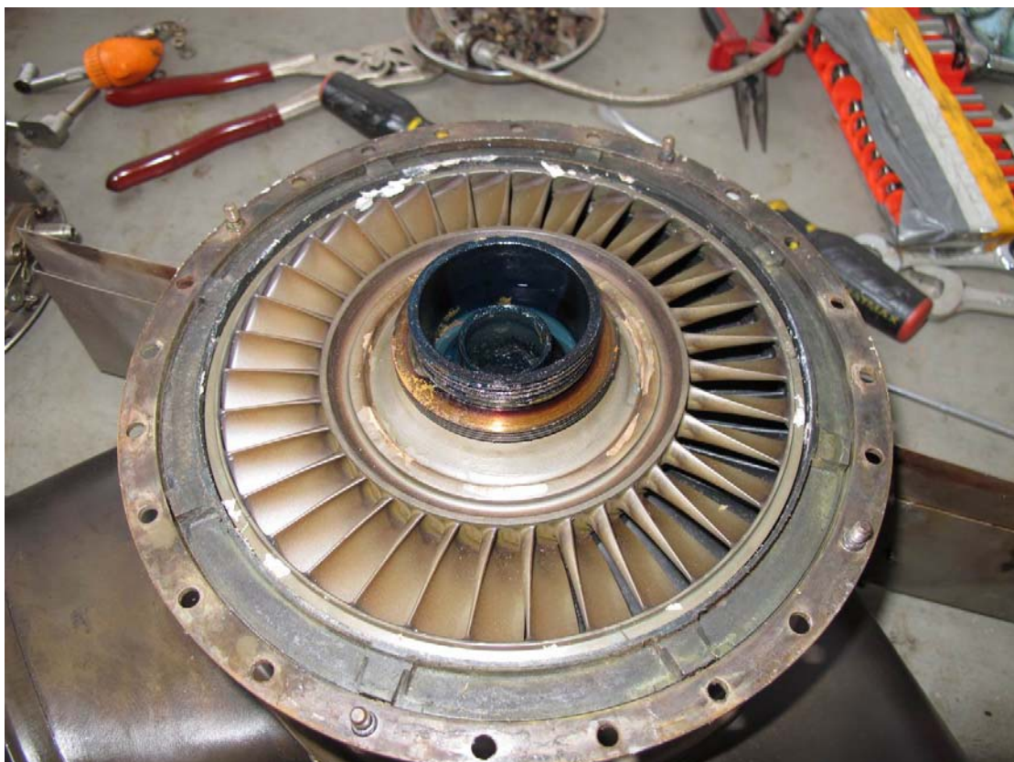
Figure 15 Third Stage Turbine Wheel
