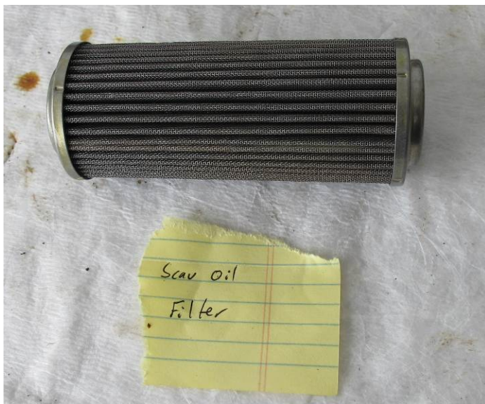
Figure 4 Scavenge Oil Filter Element
