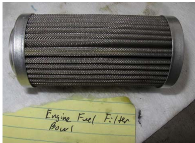
Figure 12 Fuel Pump Fuel Filter Element
