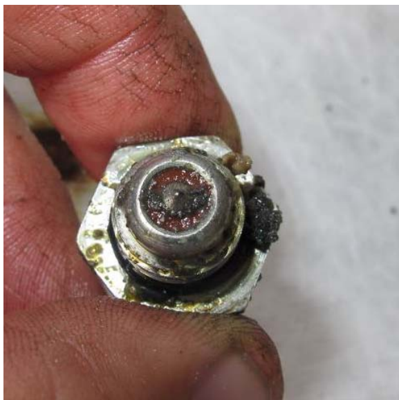
Figure 21 Top Magnetic Chip Detector
