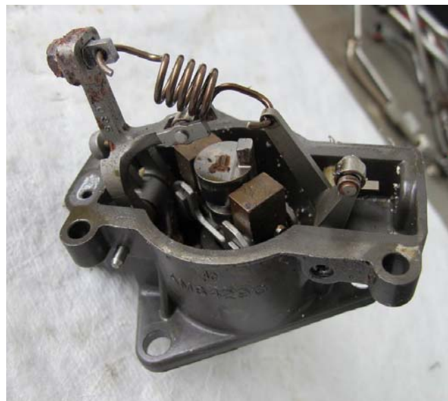
Figure 10 Power Turbine Governor Drive Body
