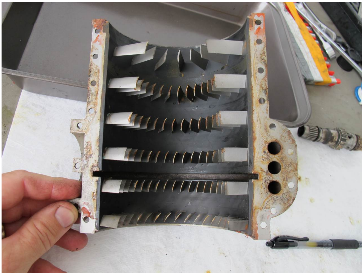
Figure 17 Compressor Case Half
