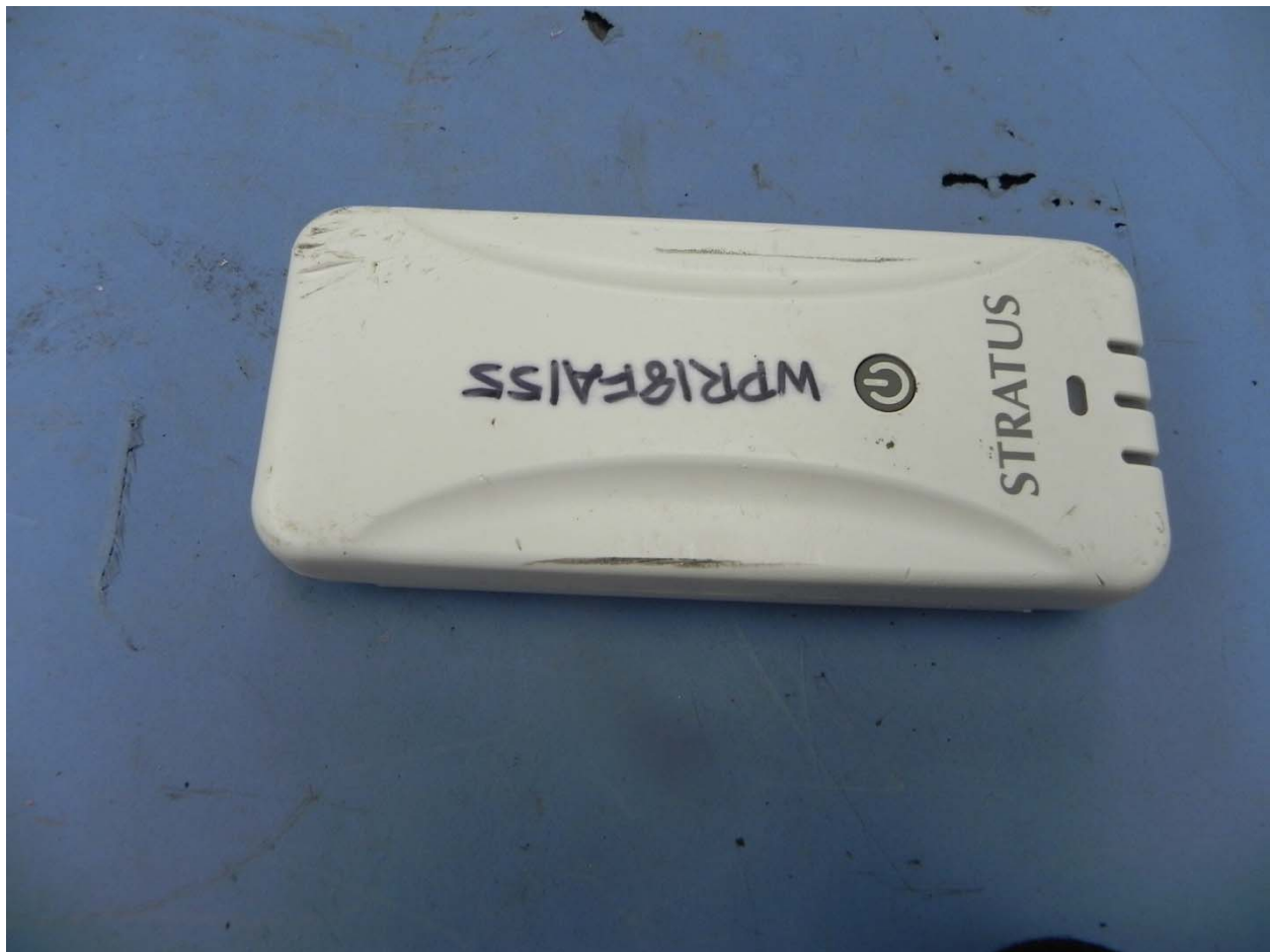
Figure 1. Photo of minor damage to Stratus PRX V2.
