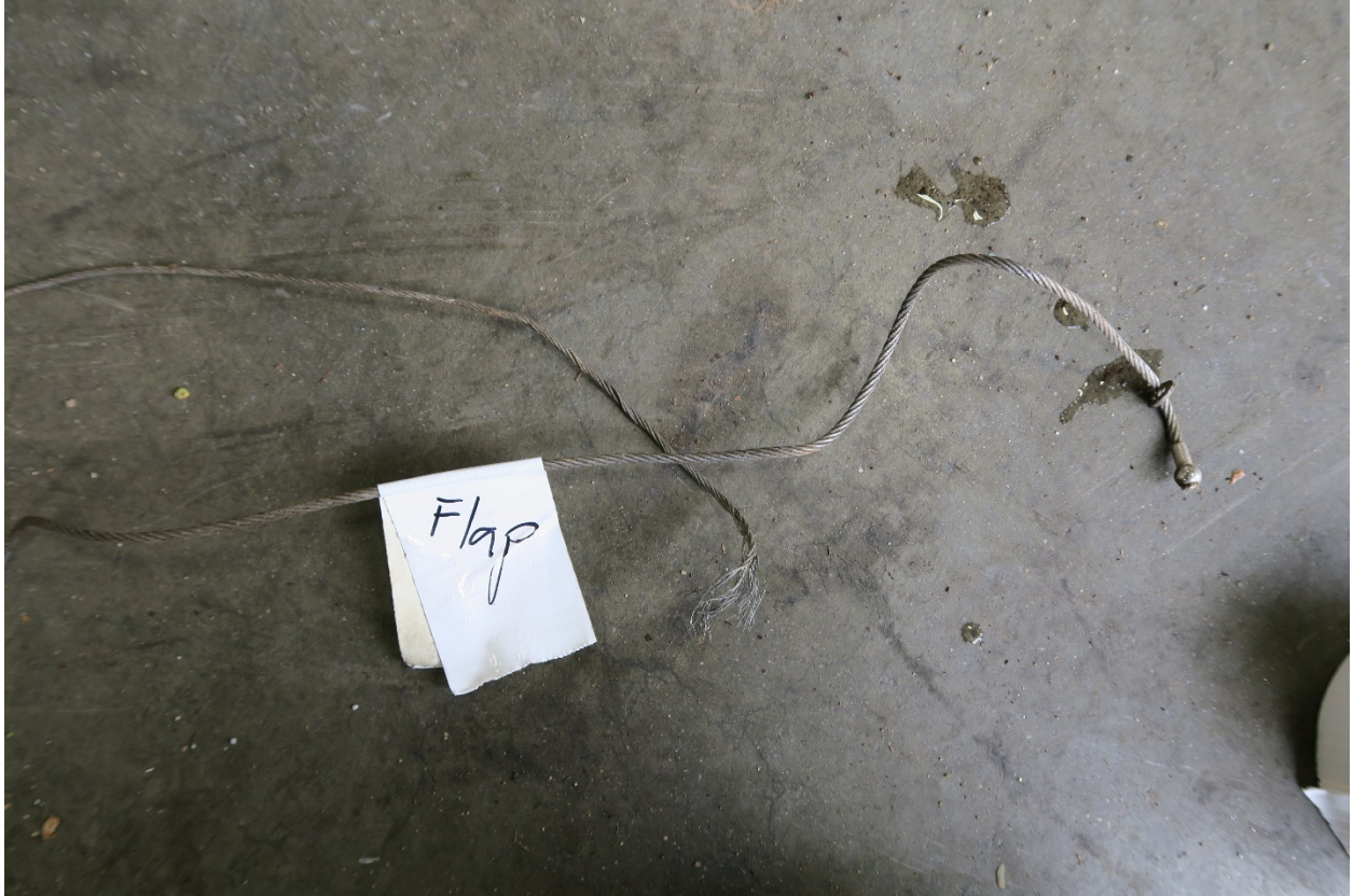
Photograph 4: Right Flap Balance and Main Cables
