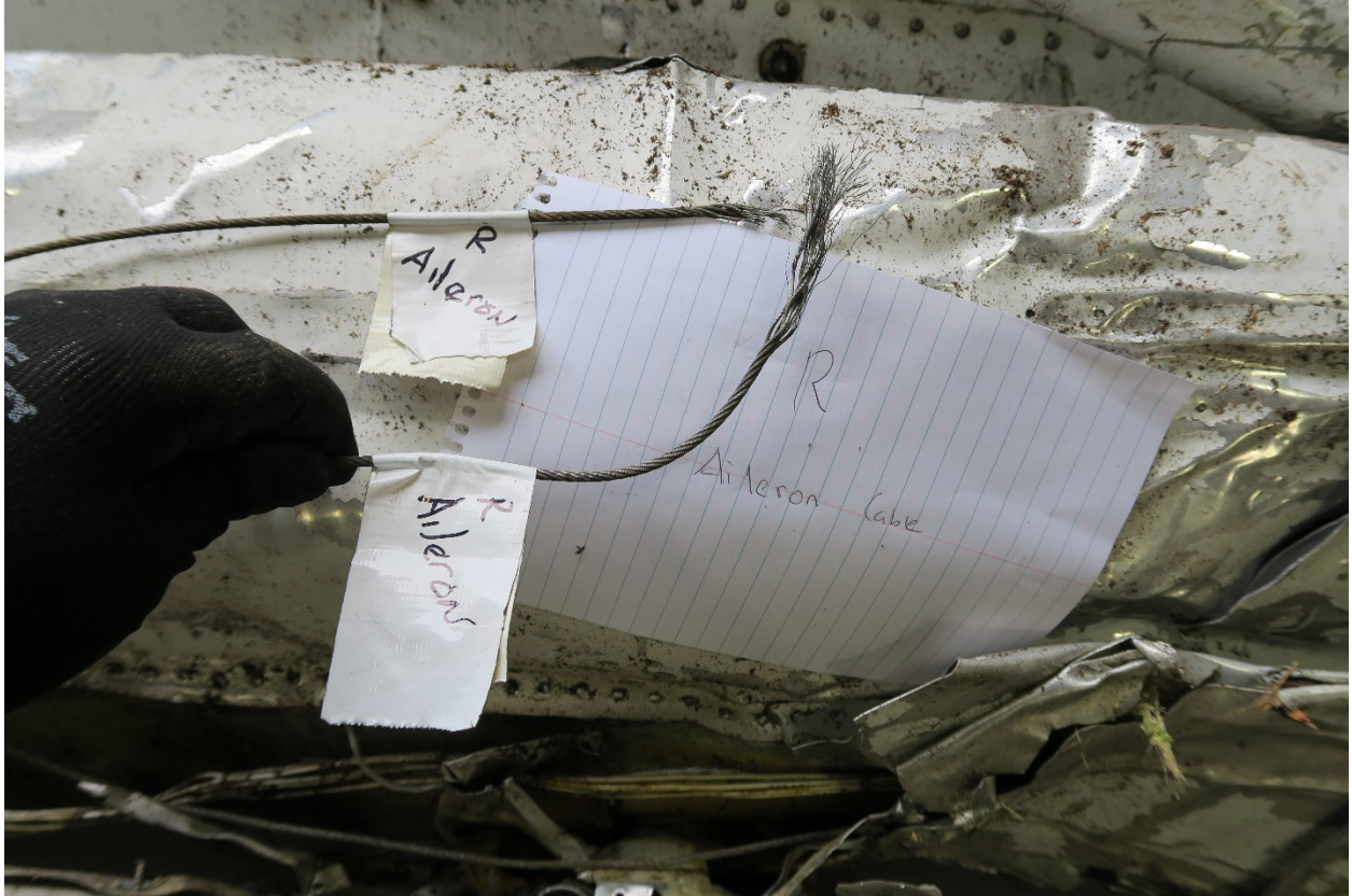
Photograph 3: Right Aileron Cable
