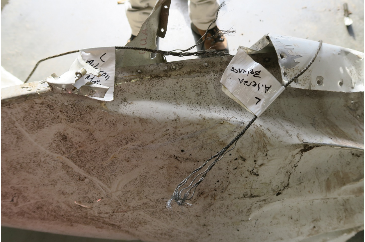
Photograph 6: Left Aileron Main and Balance Cables
