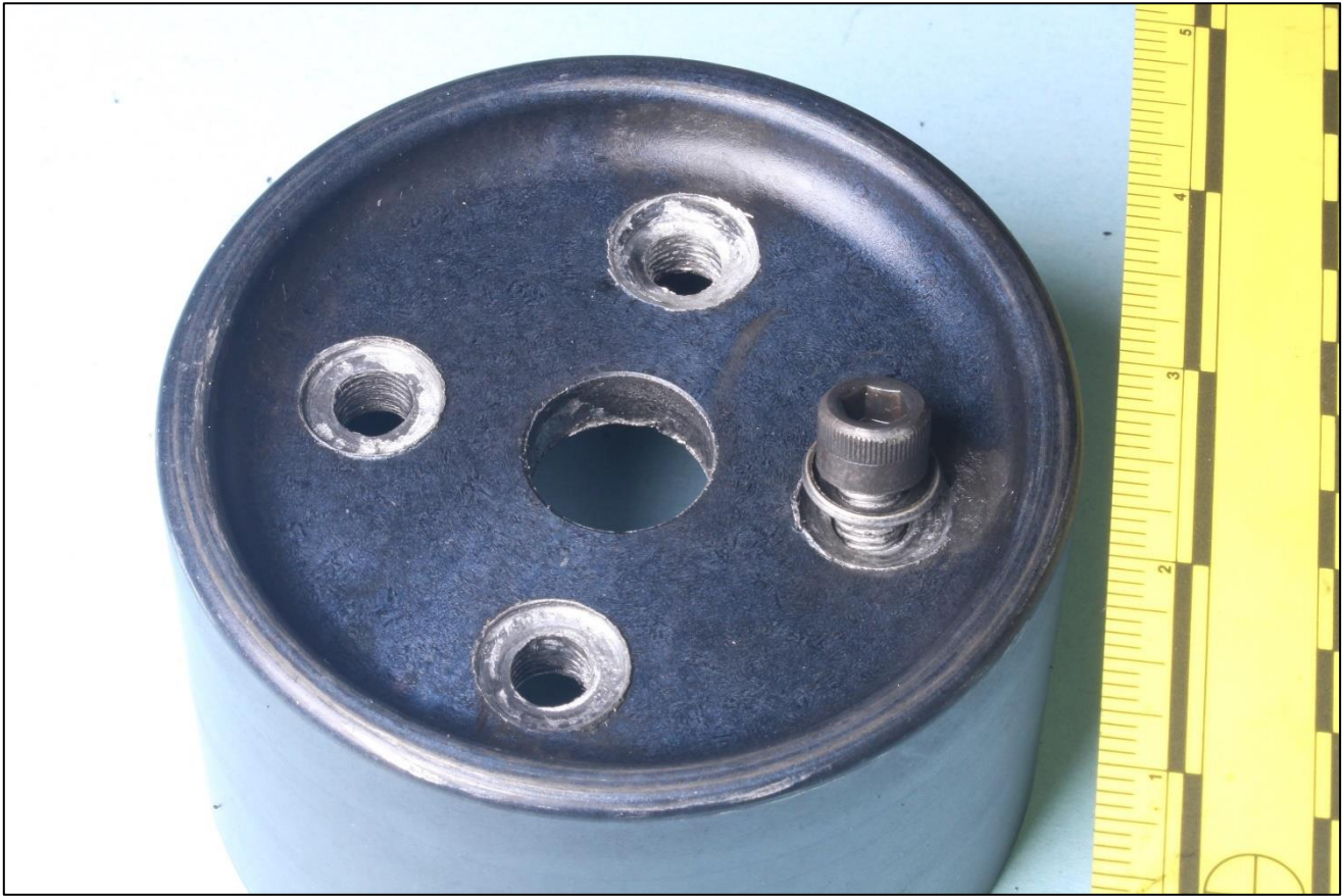
Figure 5. View of the forward face of the pulley with a trapped attachment cap screw and washer.
