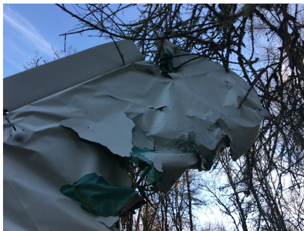
Image 6 – Impact damage on the left wing
