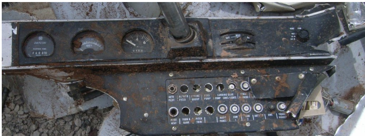
Figure 9 - Gauges and Circuit Breaker Sub-panel
