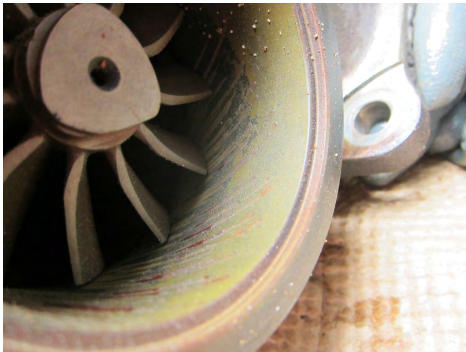
Figure 2: Spiral Streaking on the Left Turbine Housing
