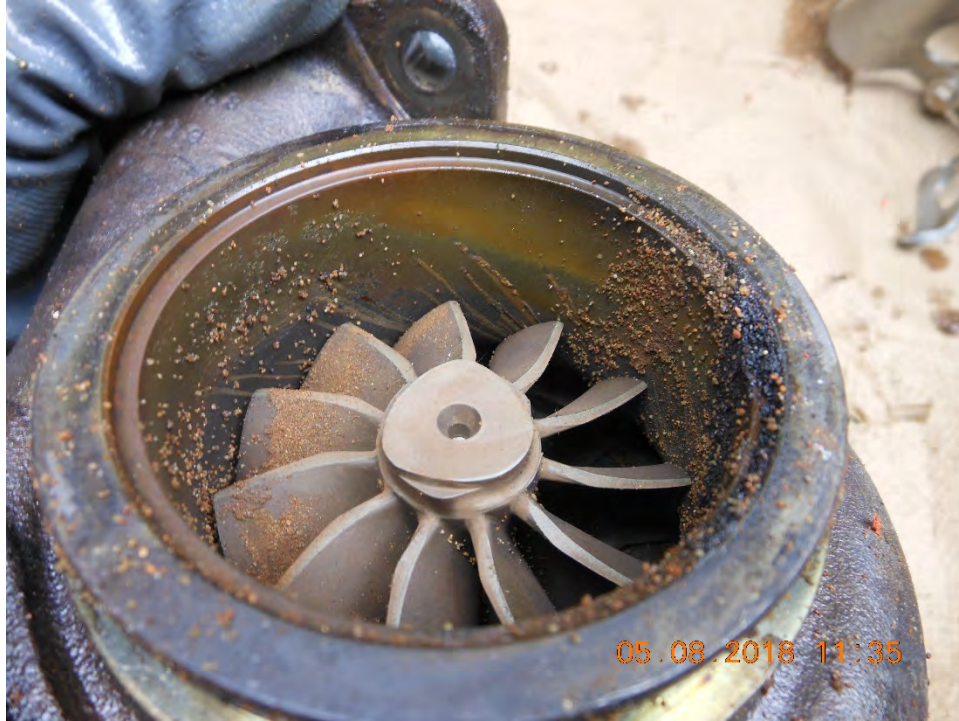
Figure 1: Spiral Streaking on the Right Turbine Housing
