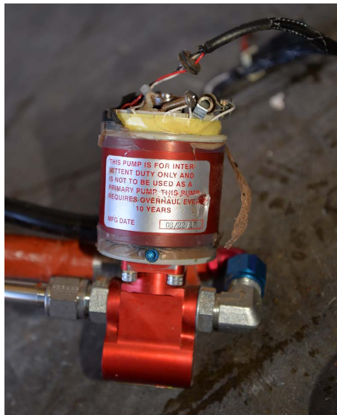
Figure 2: Electric Fuel Boost Pump
