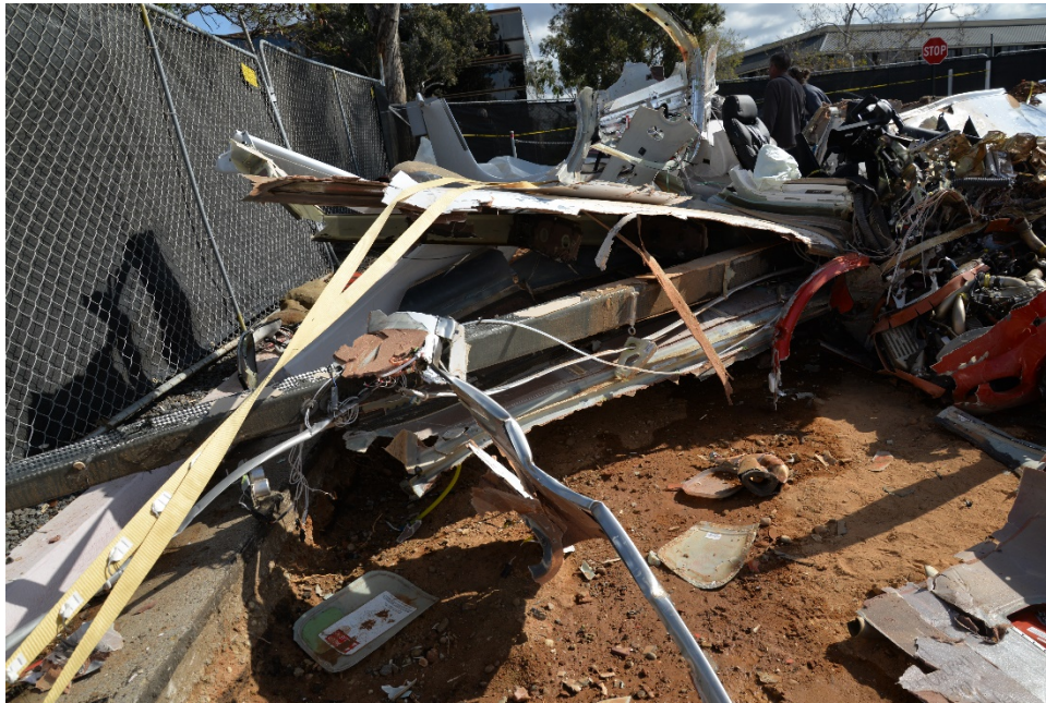
Figure 7: Right Wing Damage
