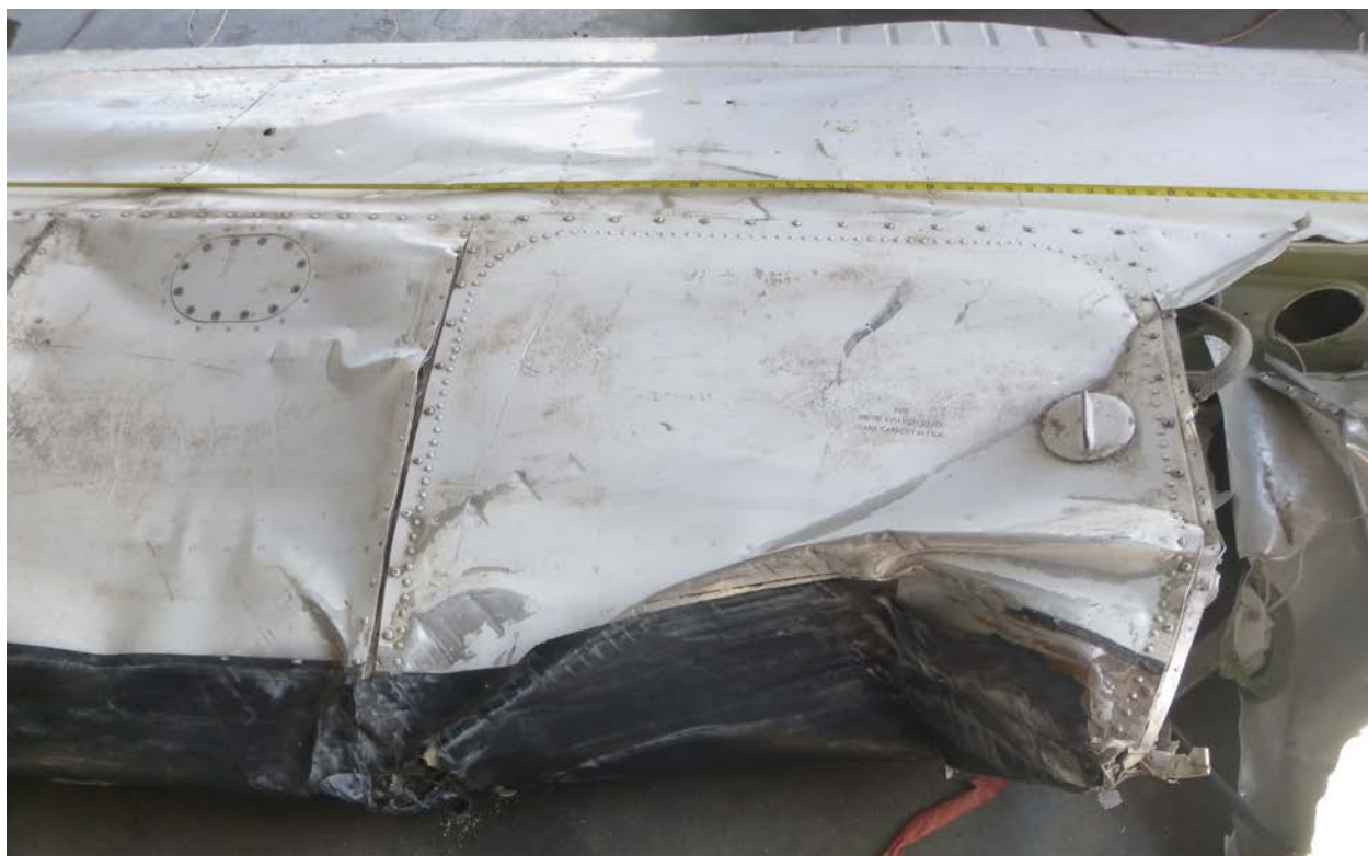
Figure 6 – Left outboard wing, upper surface
