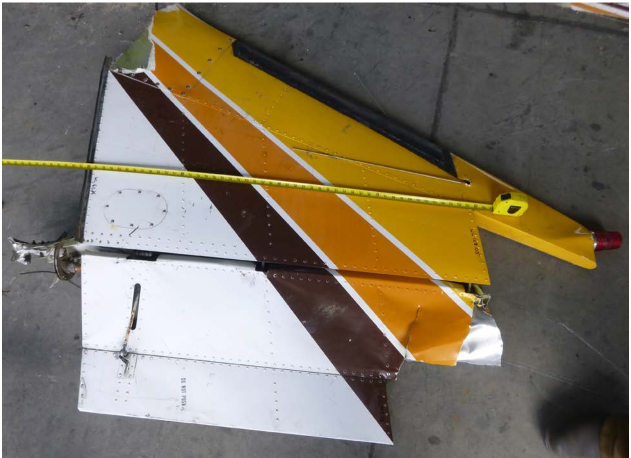
Figure 4 – Vertical stabilizer and rudder, viewed looking at left side
