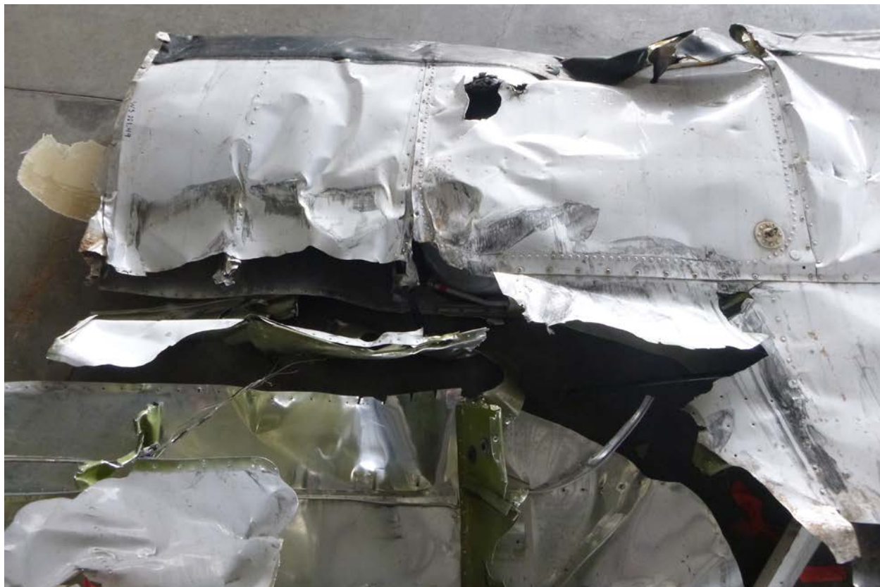
Figure 5 – Right outboard wing, lower surface
