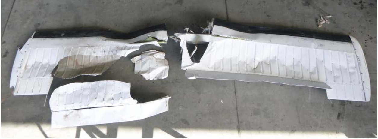
Figure 3 – Stabilator wreckage, viewed looking down at upper surface
