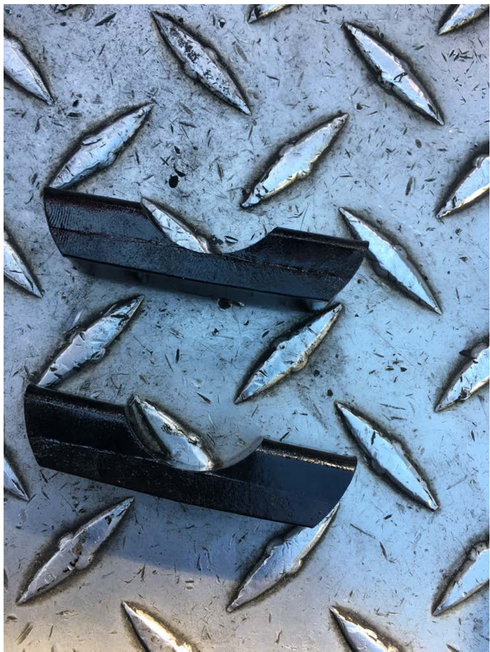
Photo 5 - Magneto bushings located in the oil screen.
