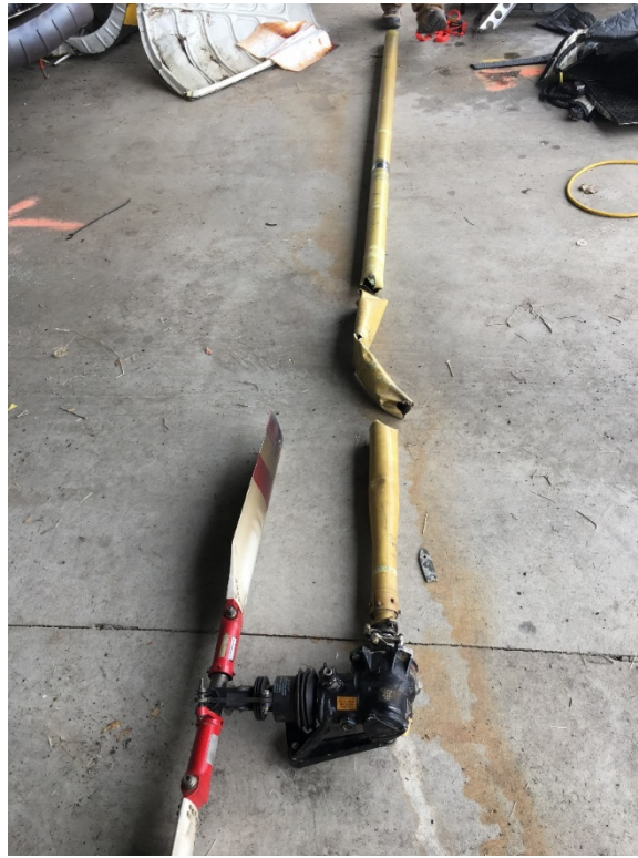
Figure 6: Tail Rotor Drive Shaft and Tail Rotor Assembly
