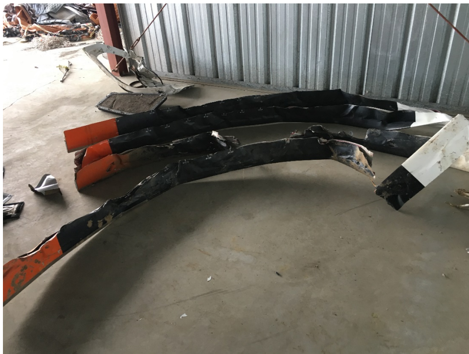
Figure 5: Four of the Five Main Rotor Blades
