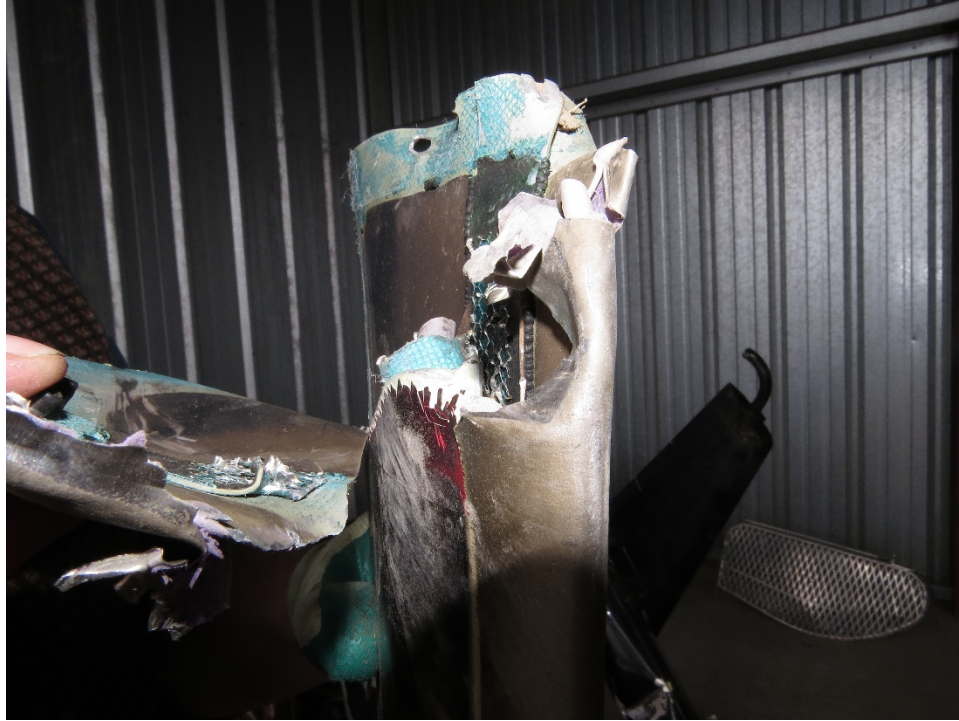
Figure 8: Leading Edge of Outboard Tail Rotor Blade
