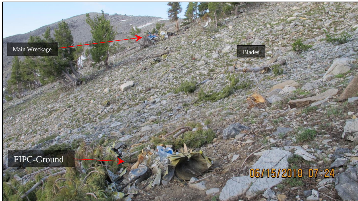
Figure 2-First Identified Point of Contact with the Ground
