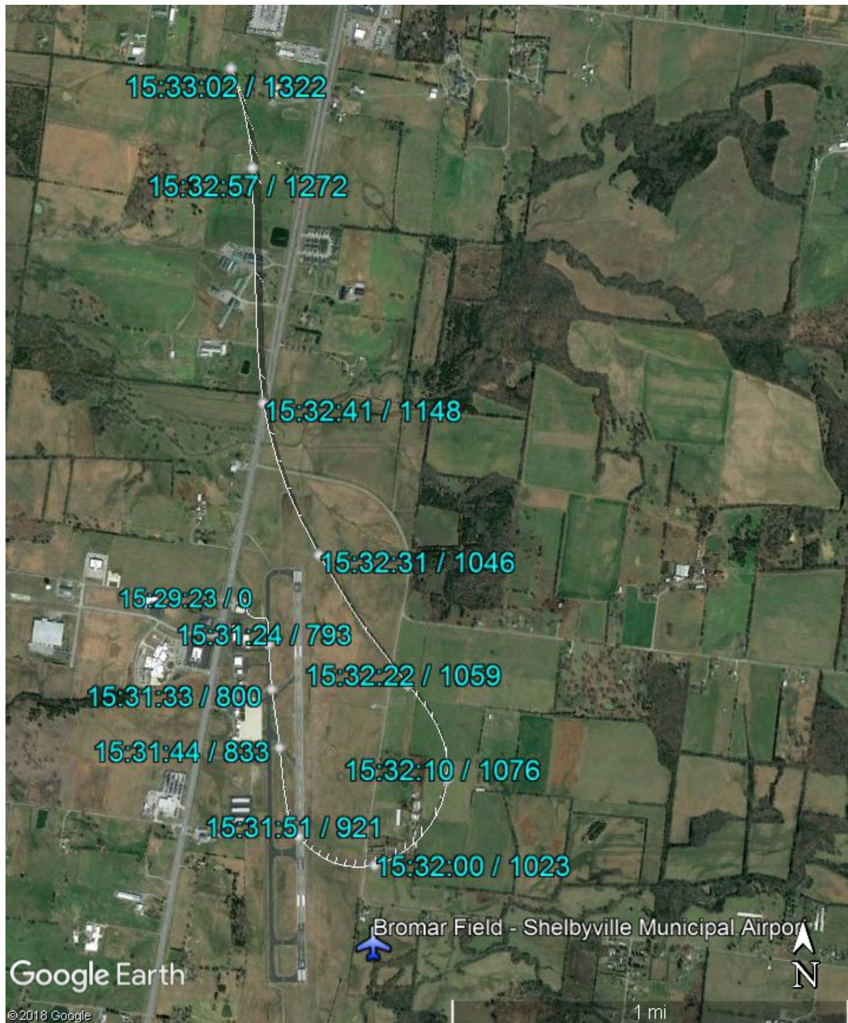
Figure 3: Accident flight take-off on December 21, 2017 from latitude, longitude, and altitude.
