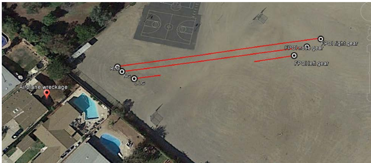
Figure 1-Landing roll on Google Earth
