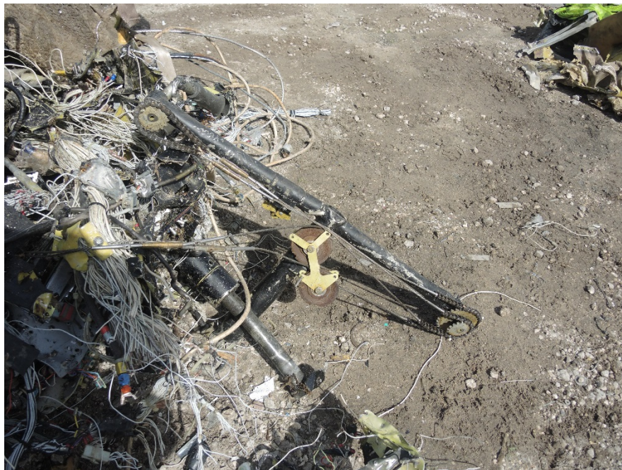
Aileron control cables
