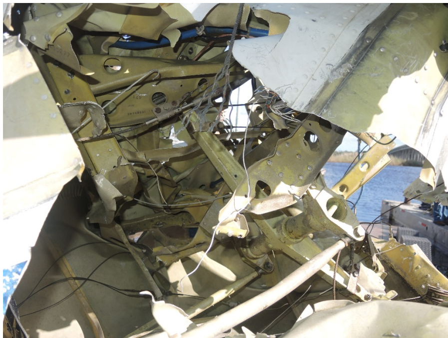
Aft elevator bellcrank
