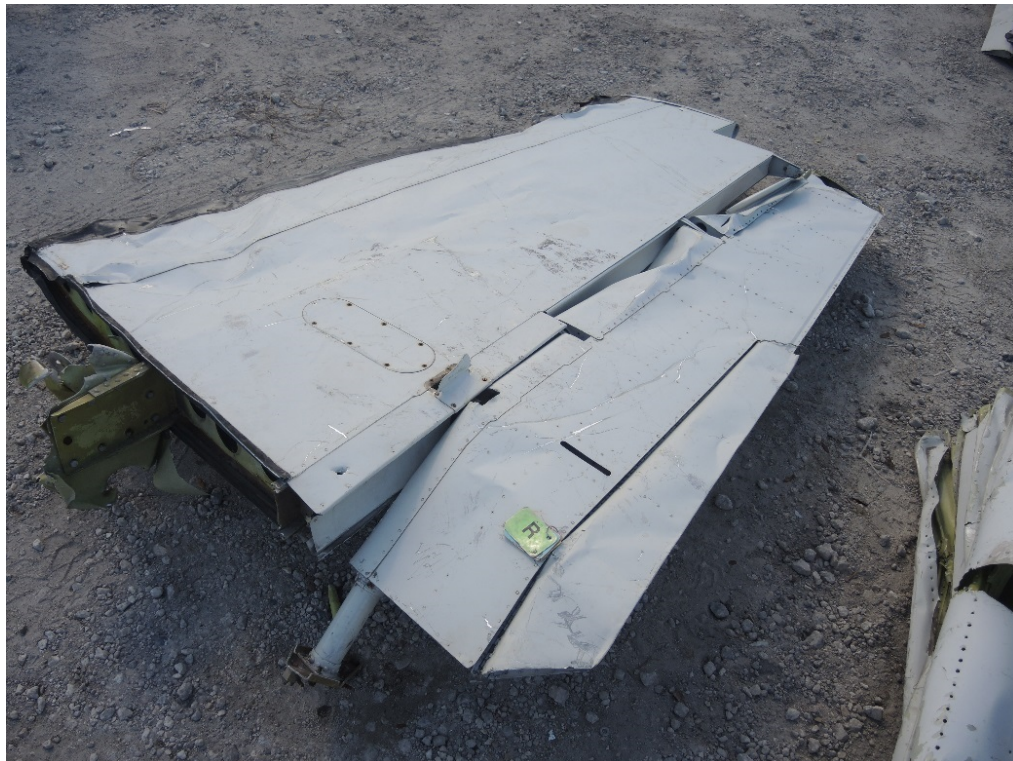
Right horizontal stabilizer and elevator
