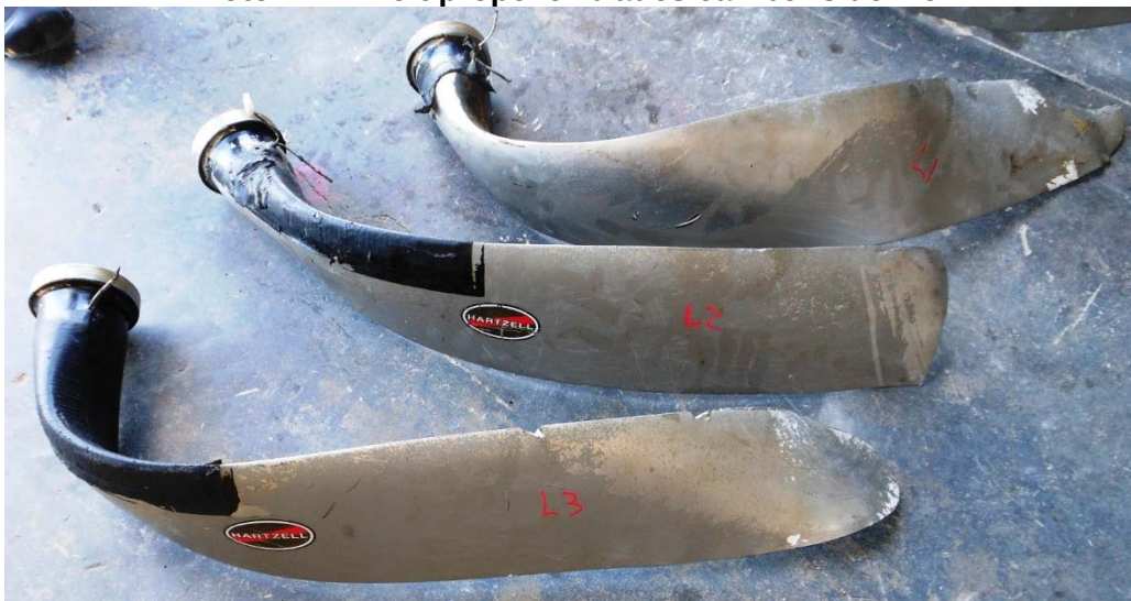
Photo #21 – Left propeller blades camber side view
