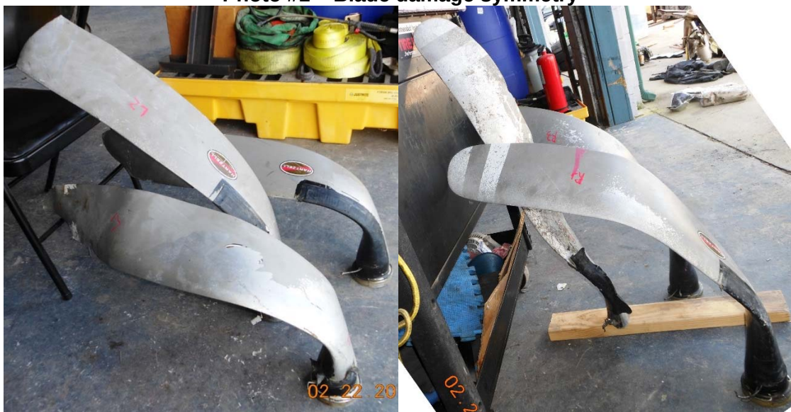
Photo #1 – Blade damage symmetry
