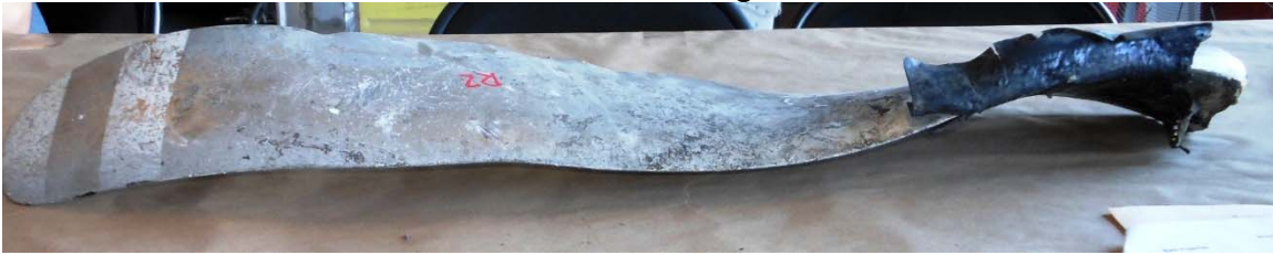
Photo #11 – Blade R2 bending characteristics
