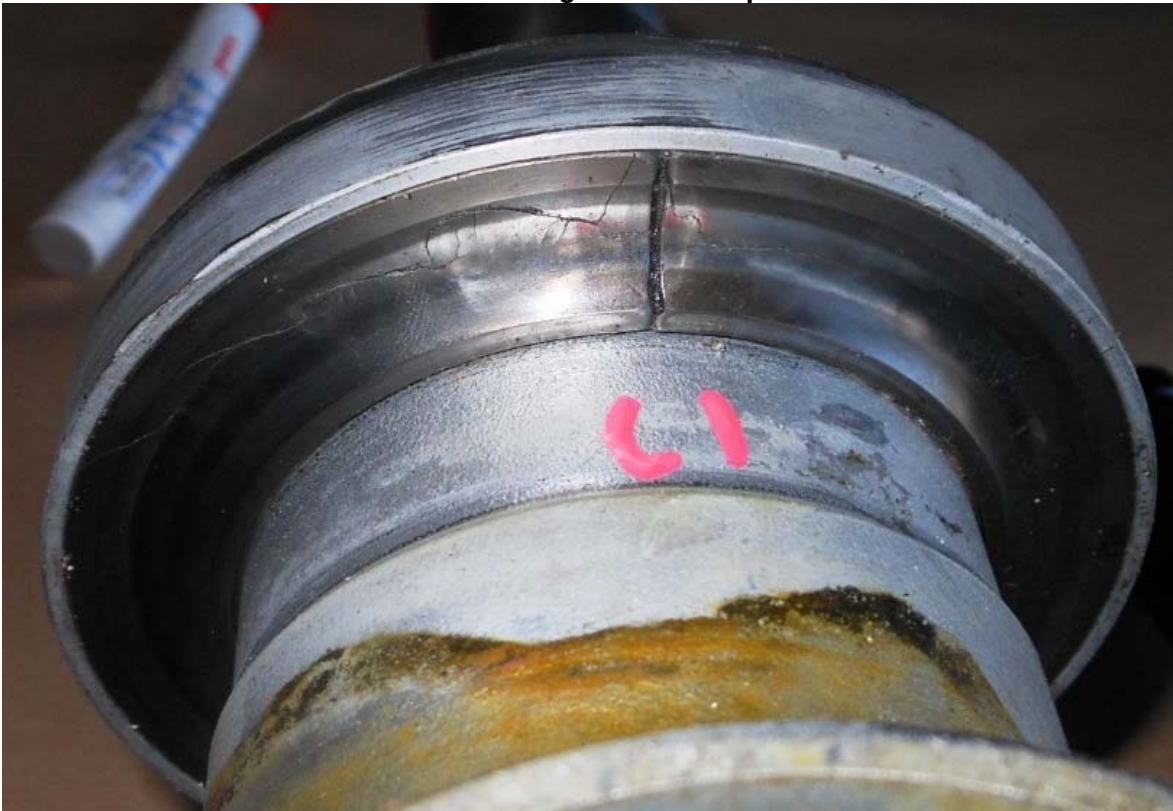
Photo #23 – Blade L1 bearing race ball imprints and cracks
