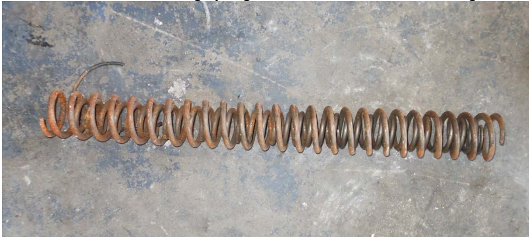
Photo #5 – Feathering spring recovered with aircraft wreckage
