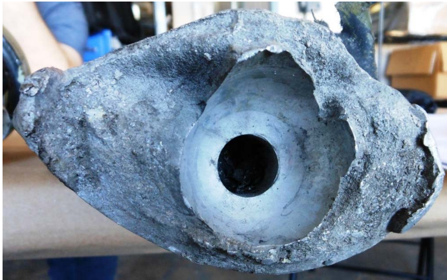
Photo #12 – Blade R2 fracture surface
