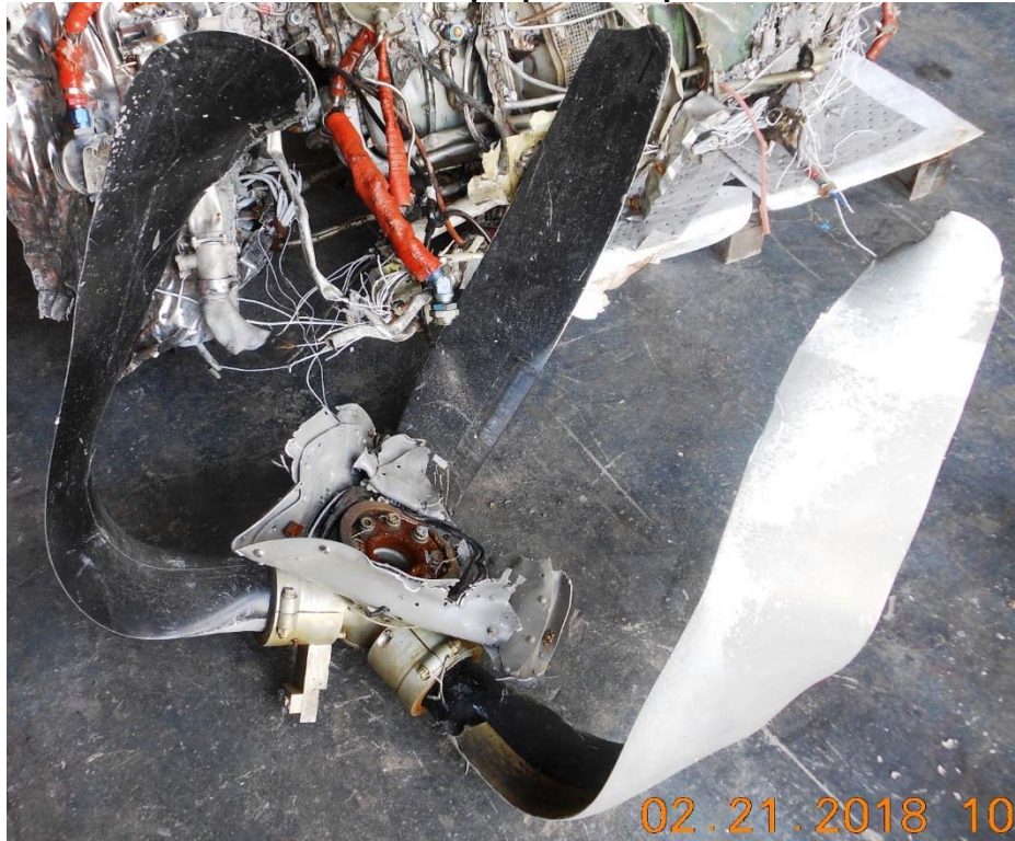
Photo #14 – Left propeller as-presented
