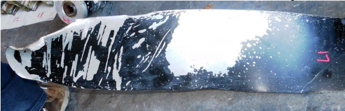
Photo #22 – Blade L1 face side chordwise/rotational scoring
