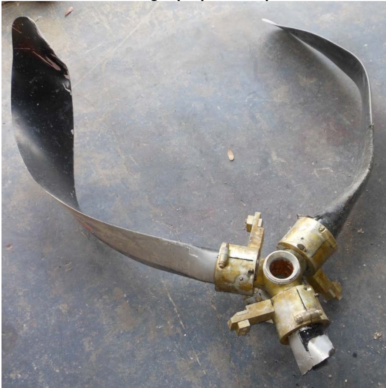
Photo #3 – Right propeller as-presented
