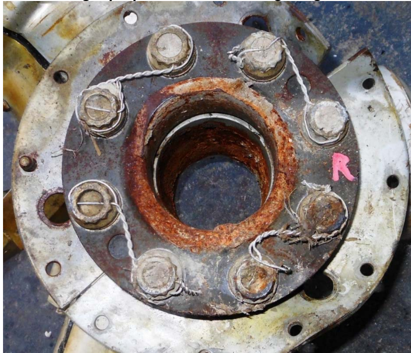
Photo #7 – Right propeller shaft mounting flange and hardware
