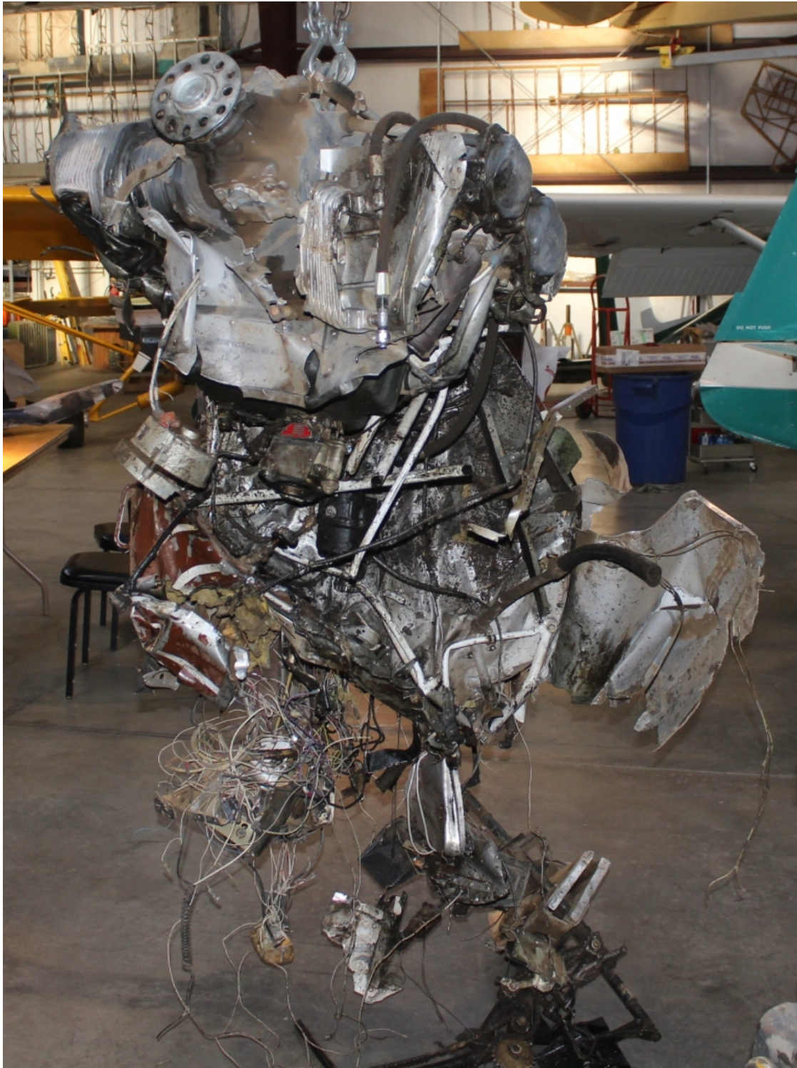
Figure 1 - Engine with Firewall and Other Components
