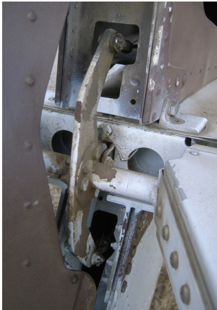
Figure 17 - Elevator Control Linkage
