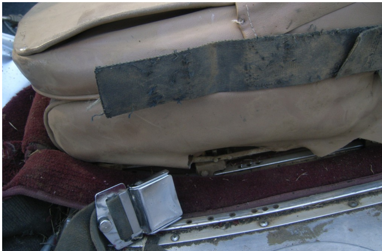
Figure 32 - Failed Stitching on Left Lap Belt
