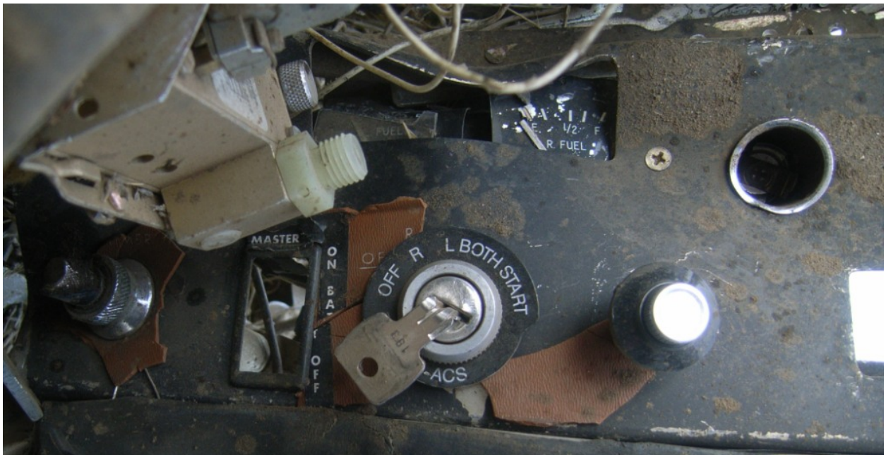
Figure 20 - Instrument Subpanel Segment
