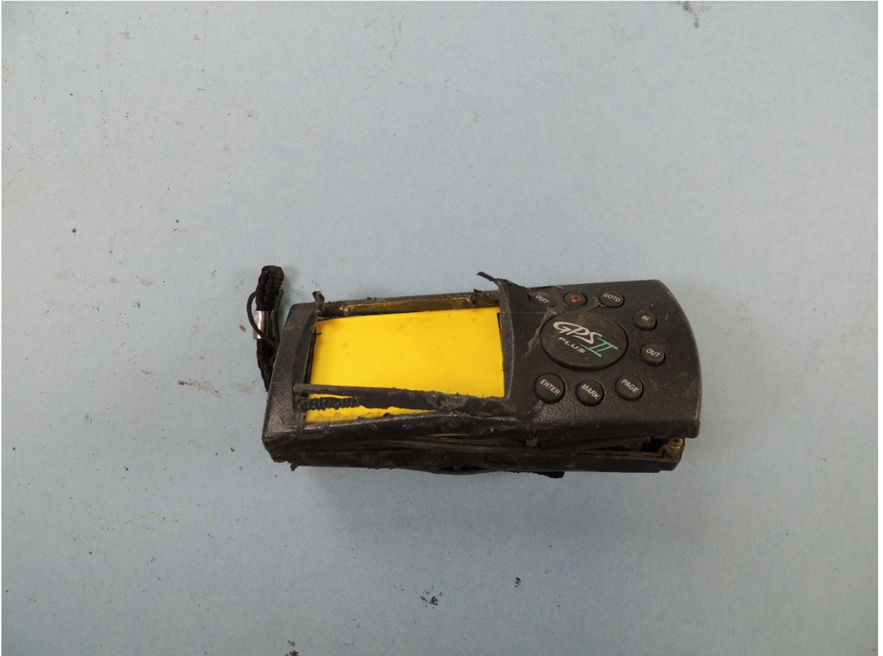
Figure 1. Damaged exterior of Garmin GPS II Plus (front side)
