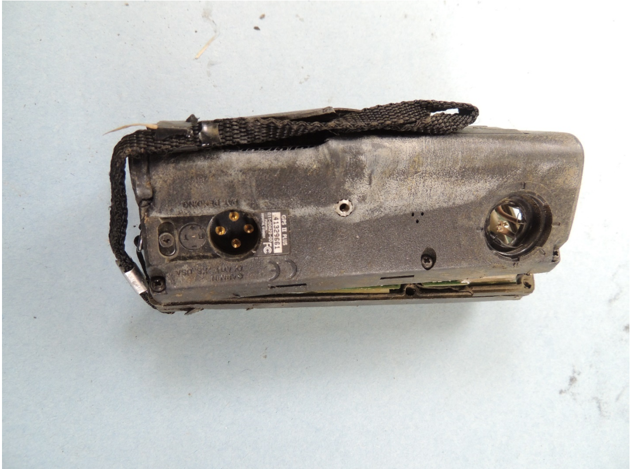
Figure 2. Damaged exterior of Garmin GPS II Plus (back side)
