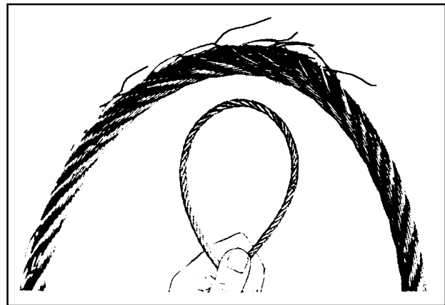
FIGURE 7-16. Cable inspection technique.
