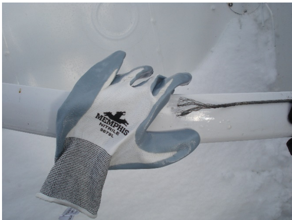
Photo 05- Left Aileron Control Cable (Piper)
