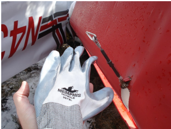
Photo 04 – Left Aileron Control Cable (Piper)
