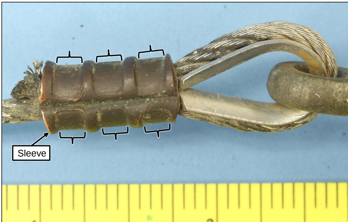
Figure 5. Close view of the cable eye at the outboard end of the left aileron balance cable. Brackets indicated crimp locations.
