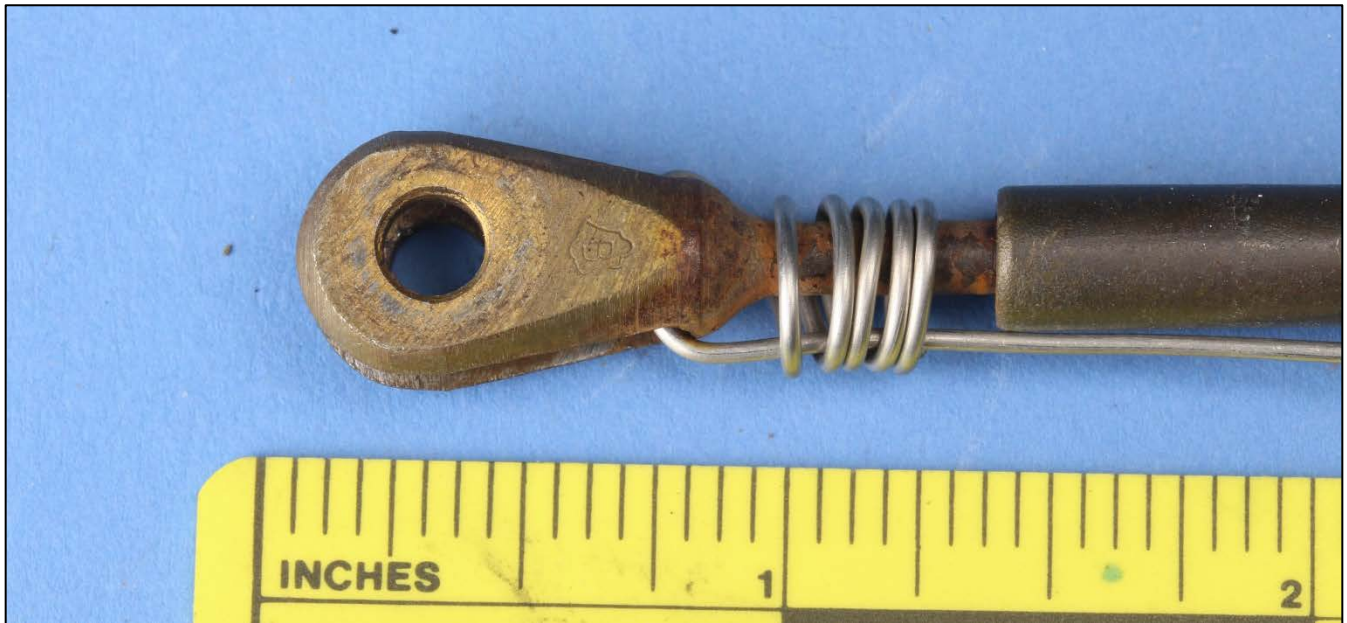
Figure 3. Closer view of the clevis end fitting on the left aileron control cable turnbuckle.
