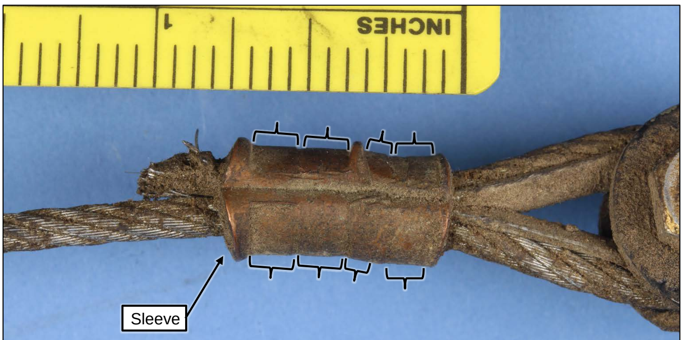
Figure 6. Close view of the sleeve at the inboard end of the left aileron control cable. Brackets indicate likely crimp locations.
