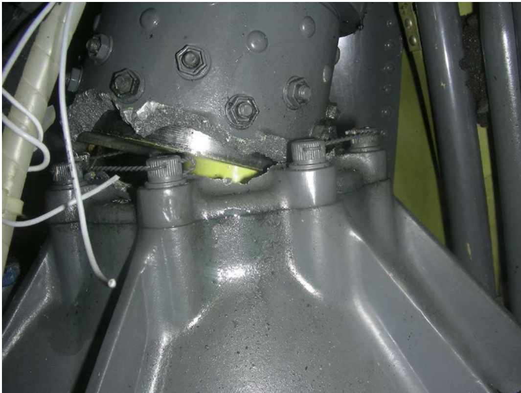
Figure 12 - main rotor gearbox fracture
