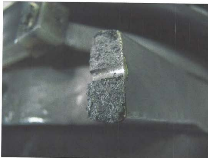
Fracture surface of Disconnect C at the swashplate arm
