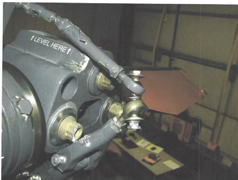
Disconnect D at the swashplate drive scissor and lower pitch control rod bolt
