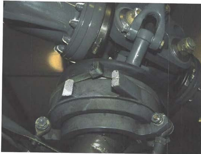
Disconnect C at the swashplate arm
