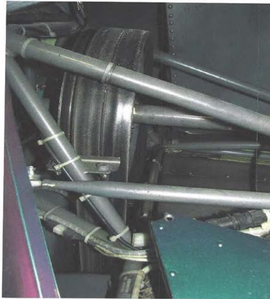
The drive belts, from the right side of the aircraft
