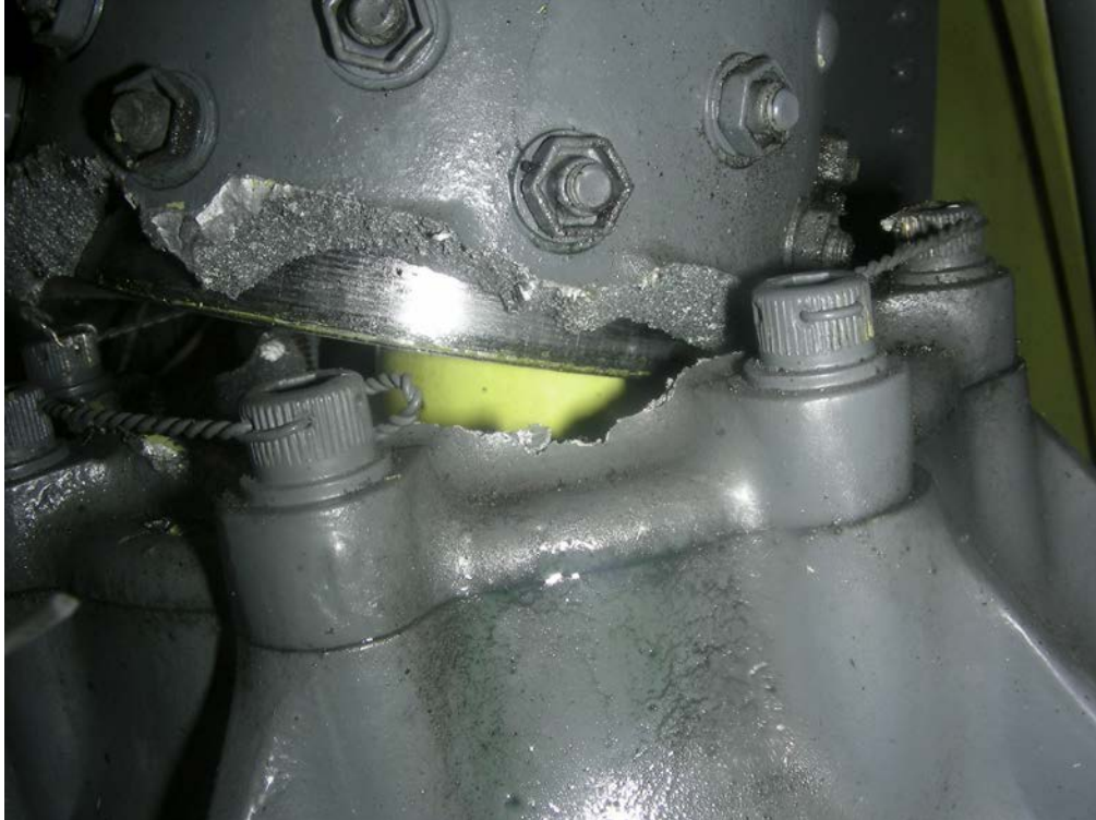
Figure 5 - photo 2 of main rotor gearbox fracture surfaces
