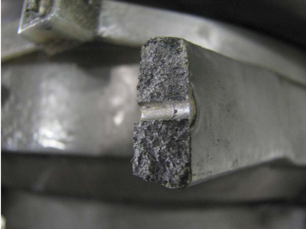
Figure 3 - photo 3 of swashplate arm fracture surface
