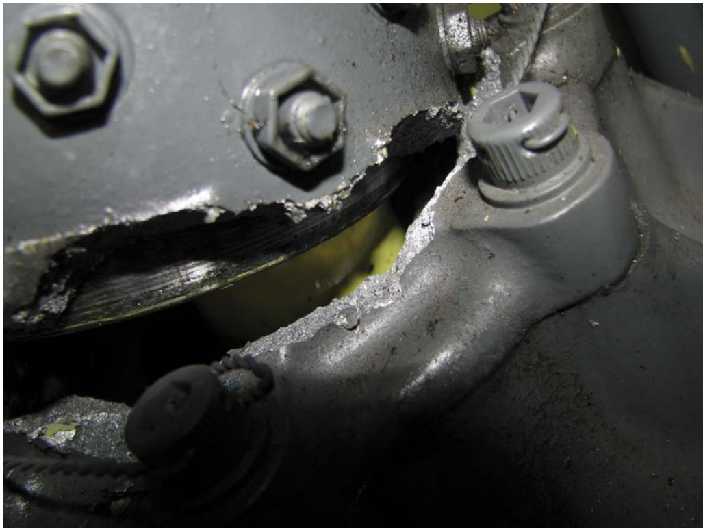
Figure 4 - photo 1 of main rotor gearbox fracture surfaces
