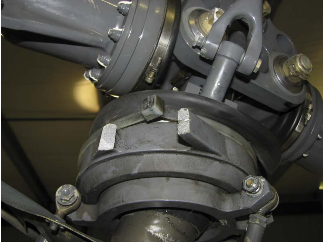
Figure 1- photo 1 of swashplate arms fracture surfaces
