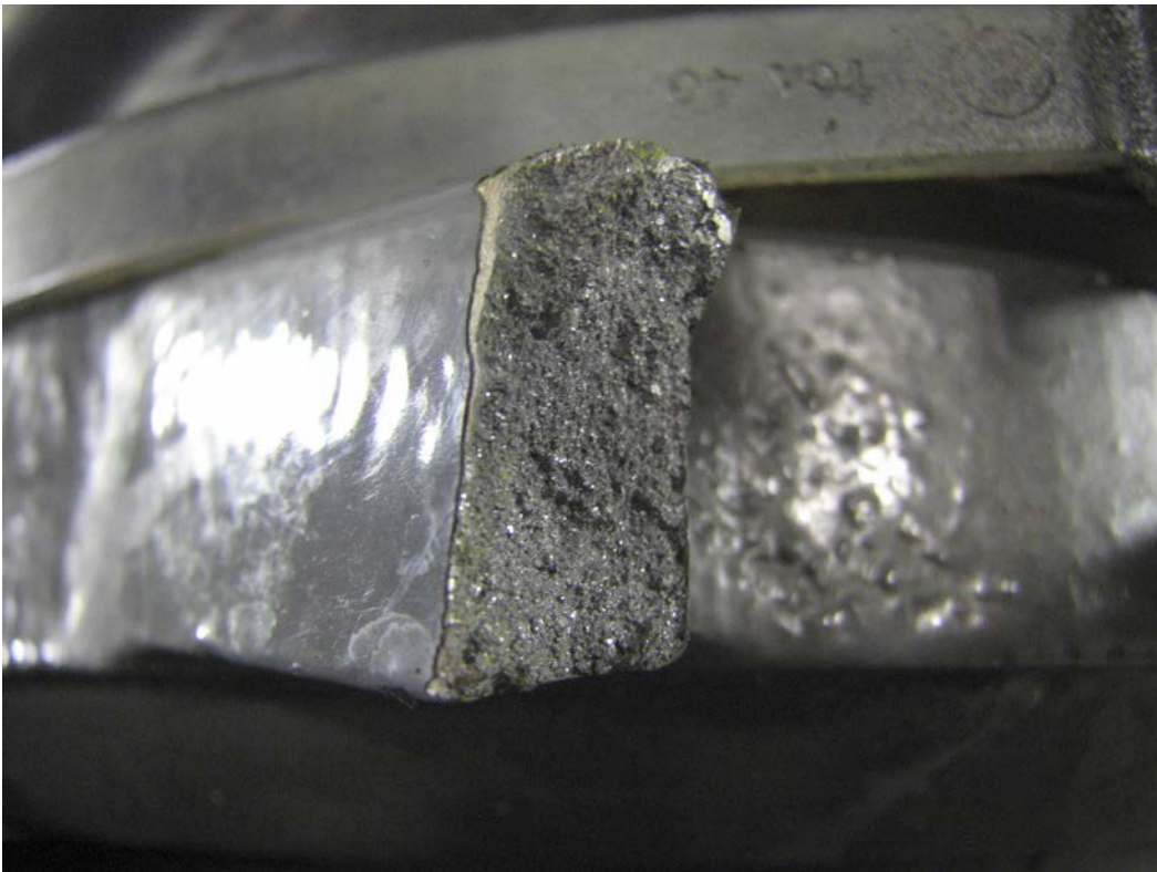
Figure 2 - photo 2 of swashplate arm fracture surface
