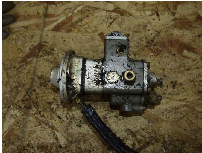
Figure 11 - engine driven fuel pump
