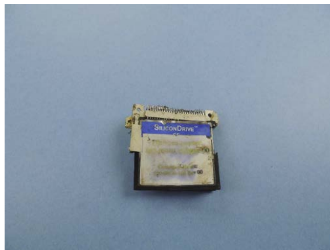
Figure 7 - top view of damaged CF memory card
