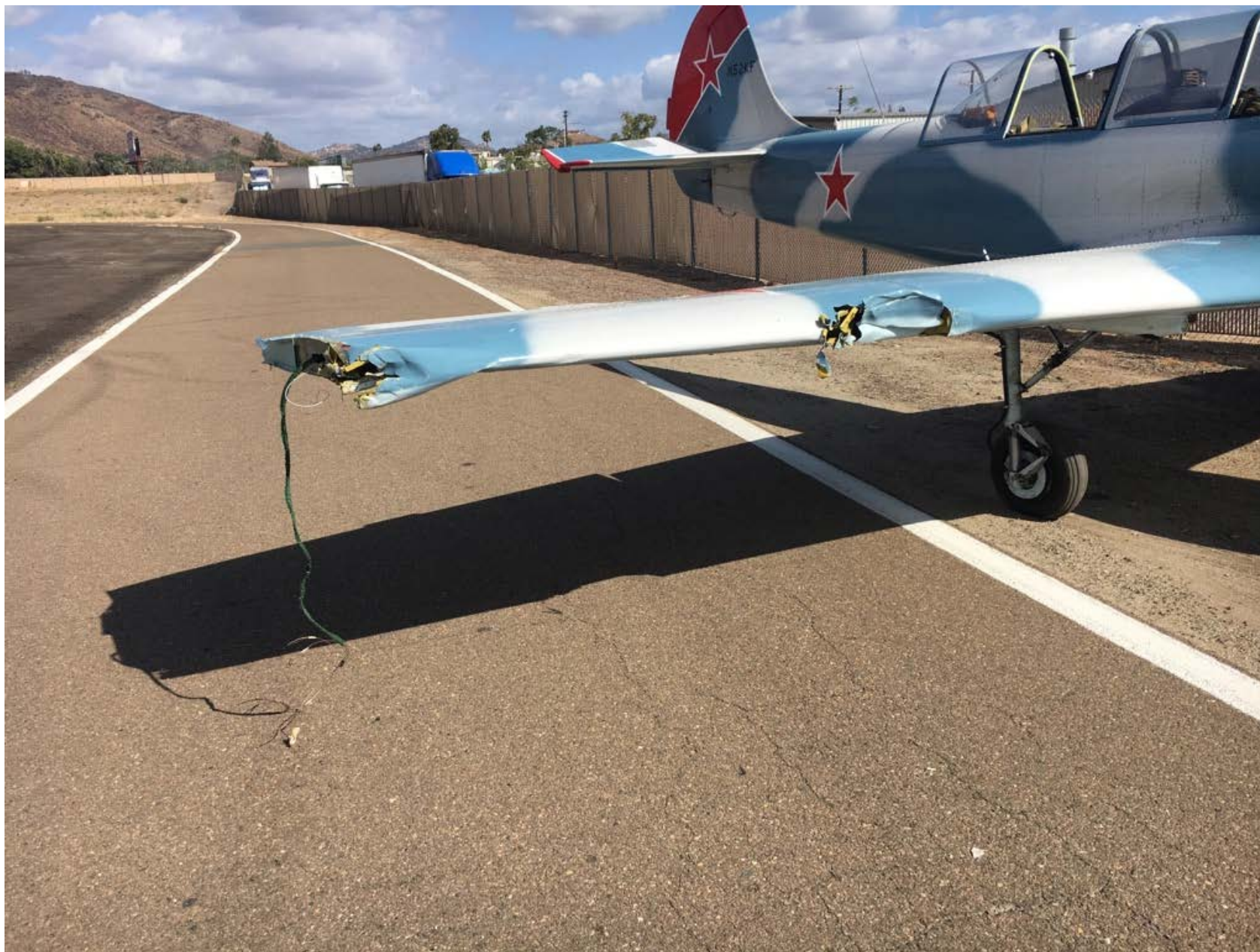
Photo 2 – Damaged left wing
