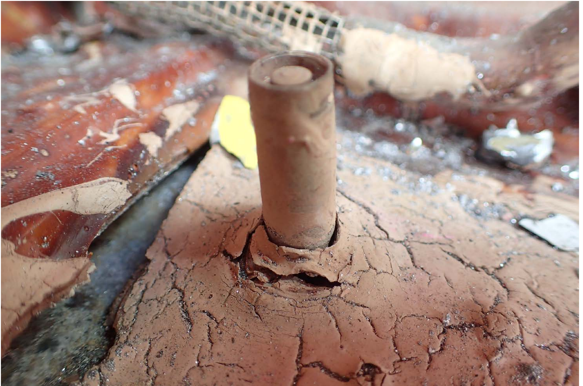
Photo 2 - Right Fuel Tank Drain Valve and Tank Breach
