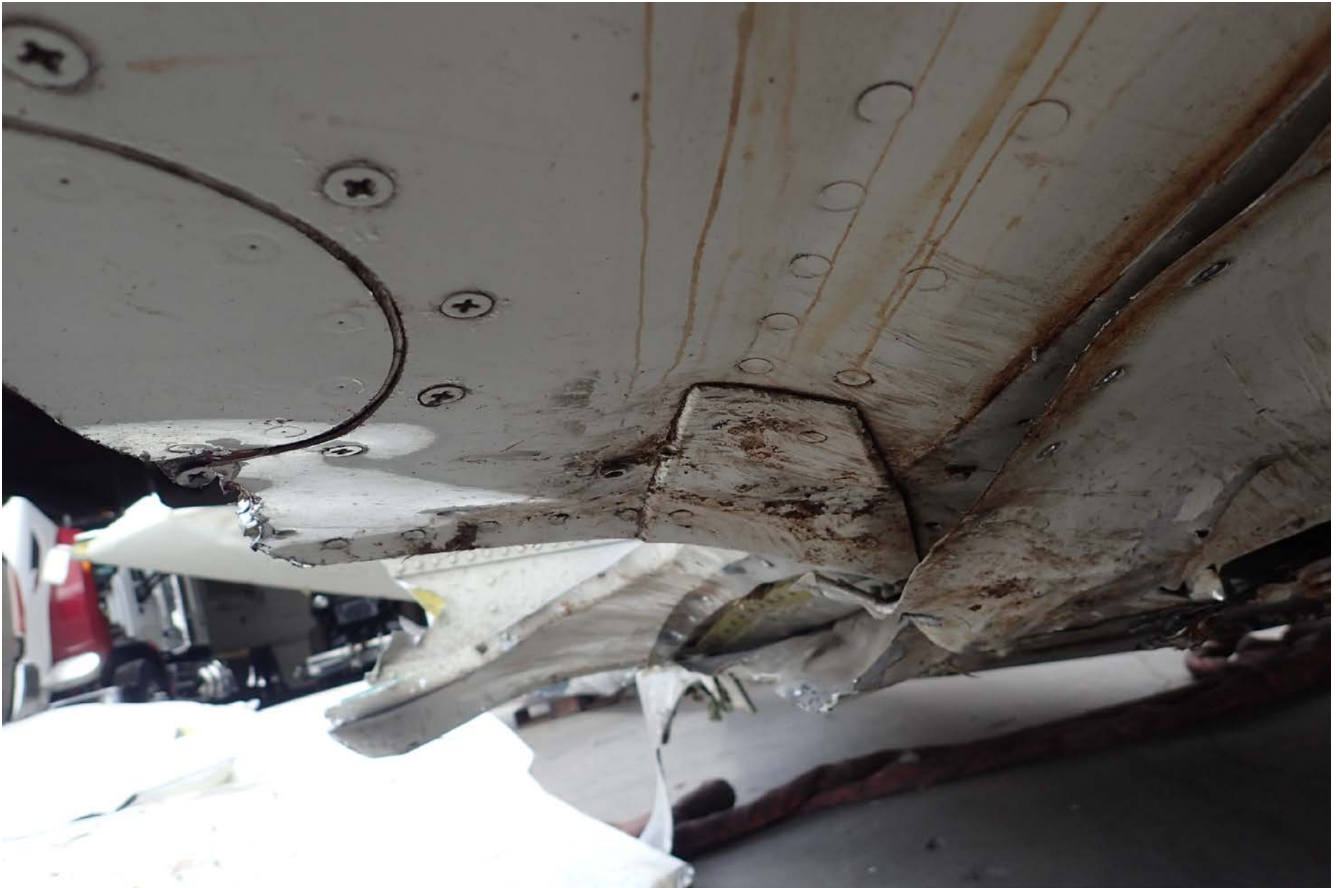
Photo 3 - Streaks Under Right Fuel Tank
