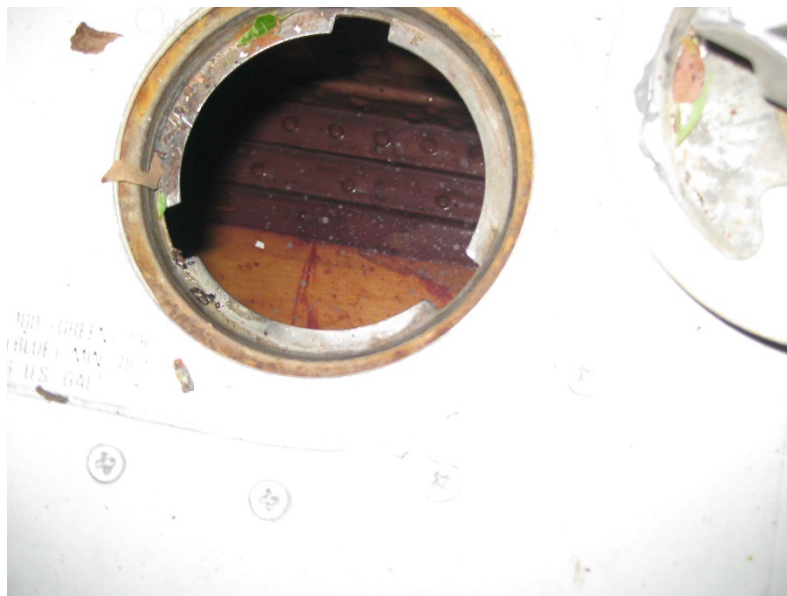
Photo 1 – Left Fuel Tank Viewed Through Filler Neck at Accident Site
