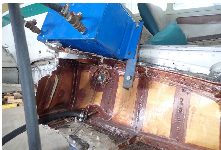
Photo 5 – Right Tank Fuel Supply for Engine Test Run
