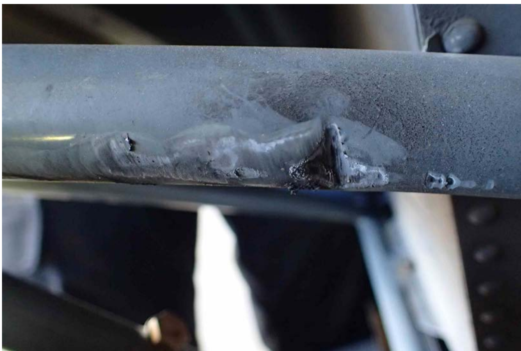
Photo 6 – Upper Frame Scoring at the Clutch Actuator
