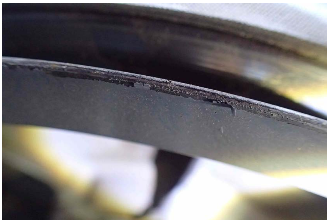
Photo 5 – Upper Sheave Radial Scoring
