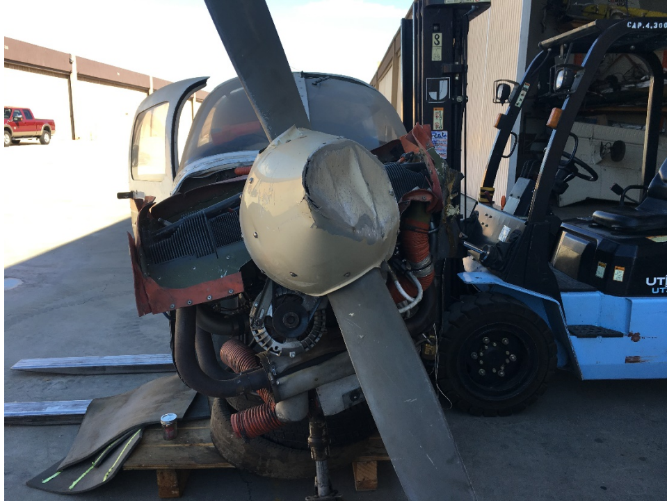
Figure 1: Impact damage to the front of Airplane
