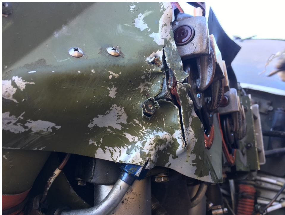
Figure 2: Impact damage to the forward section of Cylinder 2
