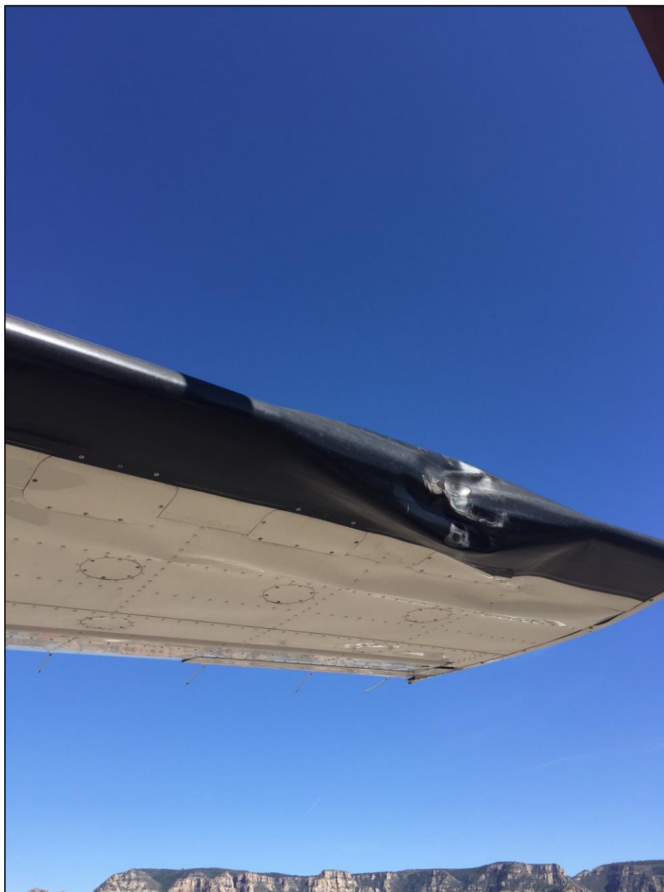
Photo 5 – Wing Leading Edge Damage
